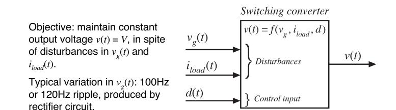
Load current variations: a significant step-change in load current, such as from 50% to 100% of rated value, may be applied.
