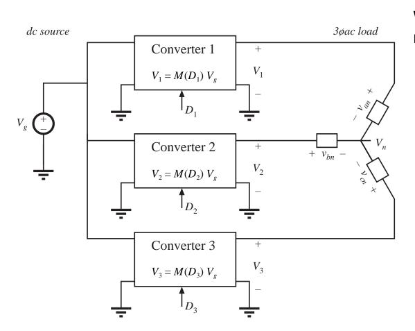
With balanced 3ø load, neutral voltage is  $V_n = \frac{1}{3} \left( V_1 + V_2 + V_3 \right)$ Phase voltages are  $V_{an} = V_1 - V_n$  $V_{bn} = V_2 - V_n$  $V_{cn} = V_3 - V_n$
