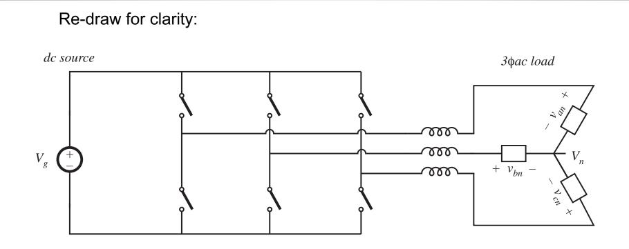
"Voltage-source inverter" or buck-derived three-phase inverter
