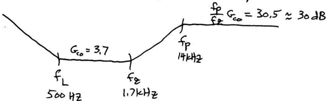
Suppose our op amp has a gain-bandwidth product of 1 MHz, so that its internal gain is
