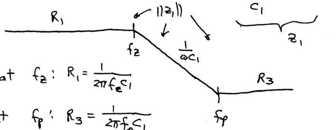
$$\text{at } f_L: R_1 = \frac{1}{2\pi f_L C_1}$$
