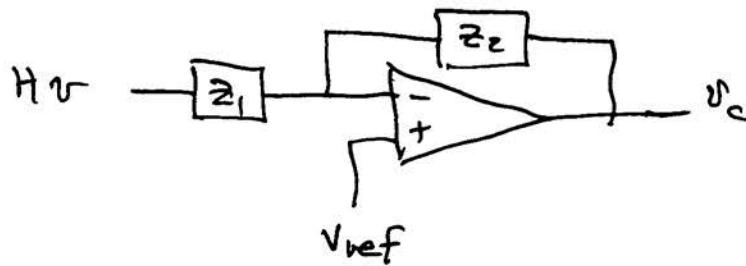
This will, however, add poles and zeroes to the transfer function from  $\hat{v}_{ref}$  to  $\hat{v}_c$ . So if  $v_{ref}(t)$  can have a significant ac component then it would be desirable to include  $Z_1$  and  $Z_2$  in the  $v_{ref}$  circuit.
