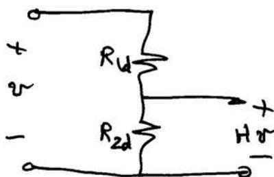
$$H = \frac{R_{2d}}{R_{1d} + R_{2d}}$$
