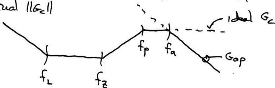
The added pole at  $f_a$  will degrade the phase margin, so we will need to account for it in our design.
