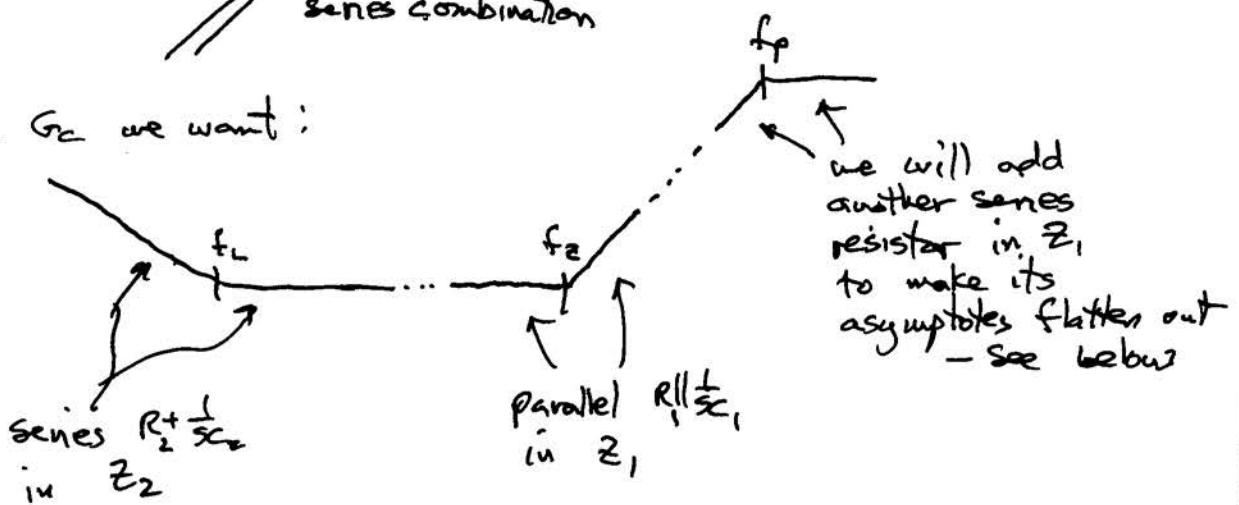
$$S_0 \quad z_2 = R_2 + \frac{1}{\omega C_2}$$
