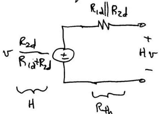
$R_{th} = R_{1d} \parallel R_{2d}$  is effectively in series with  $Z_1$
