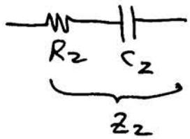
$$\text{at } f_L: R_2 = \frac{1}{2\pi f_L C_2}$$
