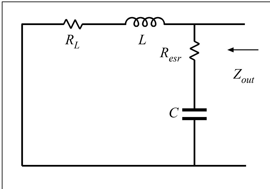
$$Z_{out}(s) = \left( R_{esr} + \frac{1}{sC} \right) \parallel (R_L + sL)$$
