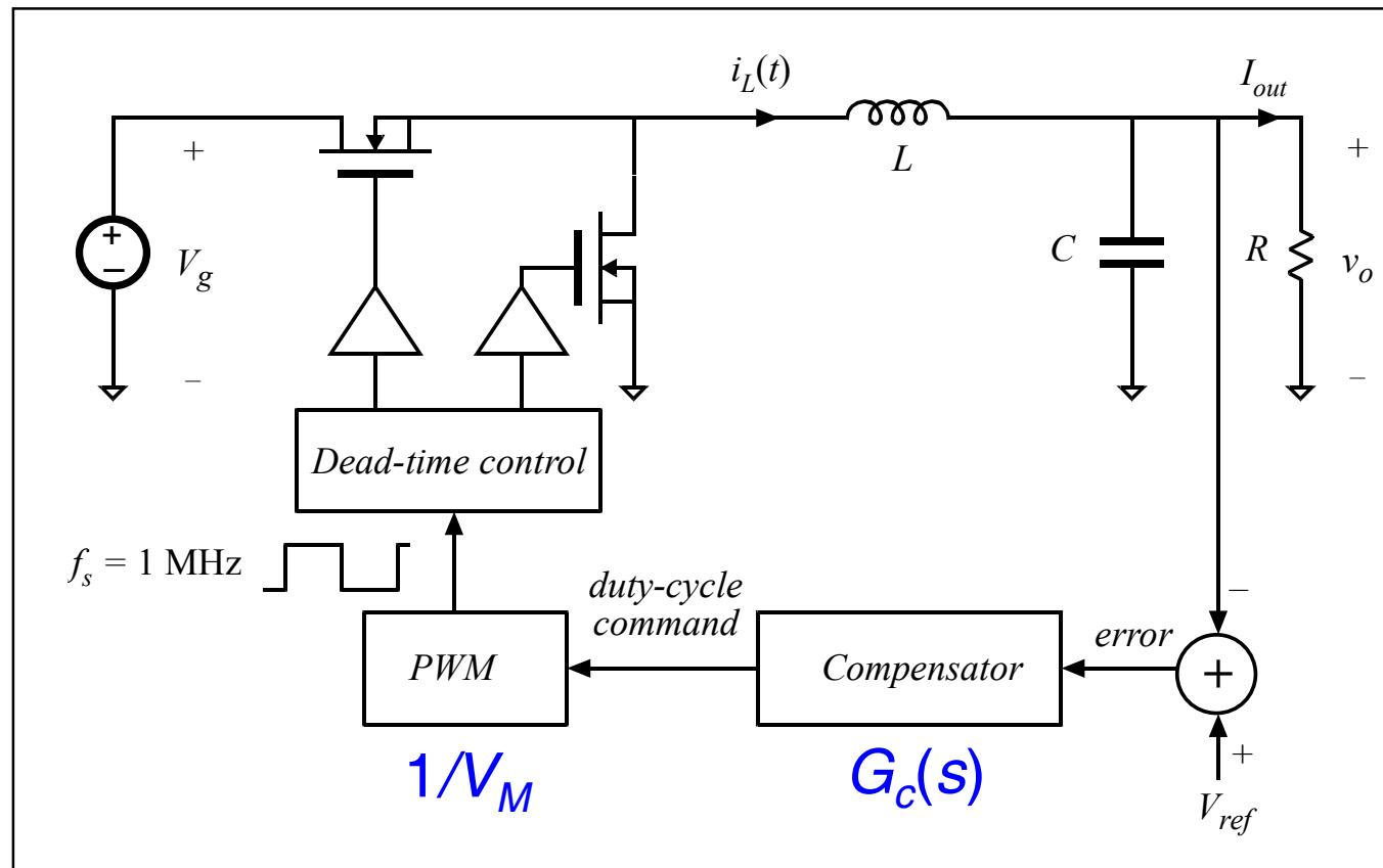
Point-of-Load Synchronous Buck Regulator
