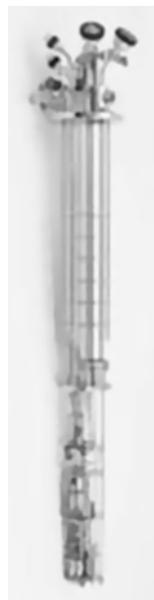
starting temperature must already have been lowered to 1 K by precooling. During operation,  $^3\text{He}$  atoms from the upper concentrated phase are dissolved continuously in the lower, much more diluted phase. In many ways this scheme resembles a regular evaporation process, in which the upper phase corresponds to the liquid and the lower phase to the vapor. As the final result, a continuous cooling of liquid helium is achieved.
