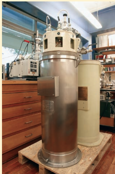
■ FIGURE 13.29 Prototype 15 kVA partial core superconducting power transformer. (Photo courtesy of Department of Electrical and Computer Engineering, University of Canterbury.)
