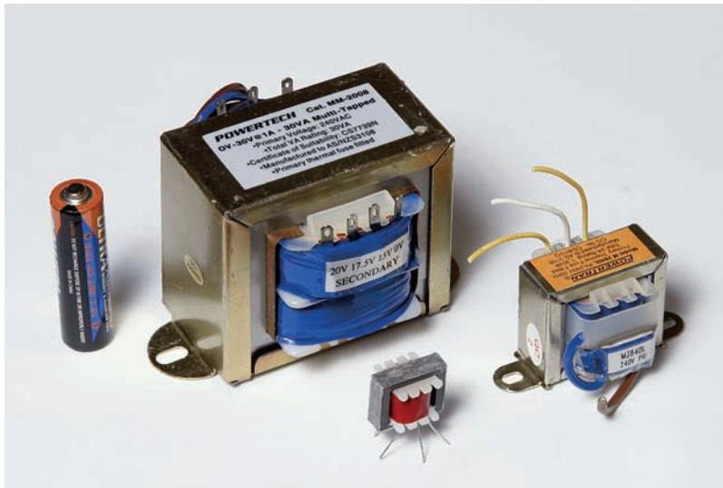
■ FIGURE 13.15 A selection of small transformers for use in electronic applications; the AA battery is shown for scale only.
