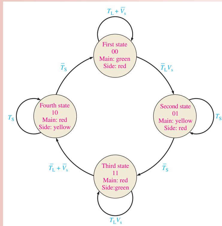
**FIGURE 6-63** State diagram for the traffic signal control.
