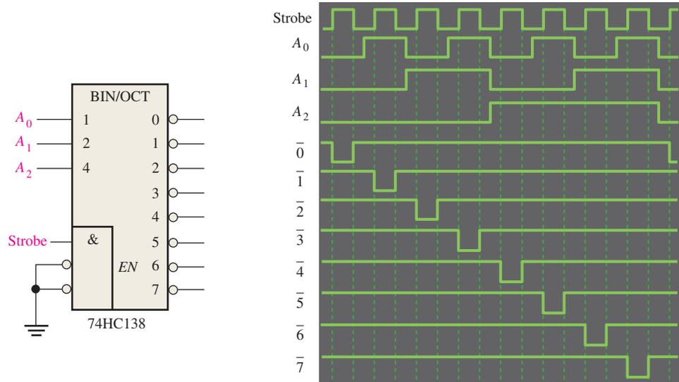
**FIGURE 6–62** Application of a strobe waveform to eliminate glitches on decoder outputs.
