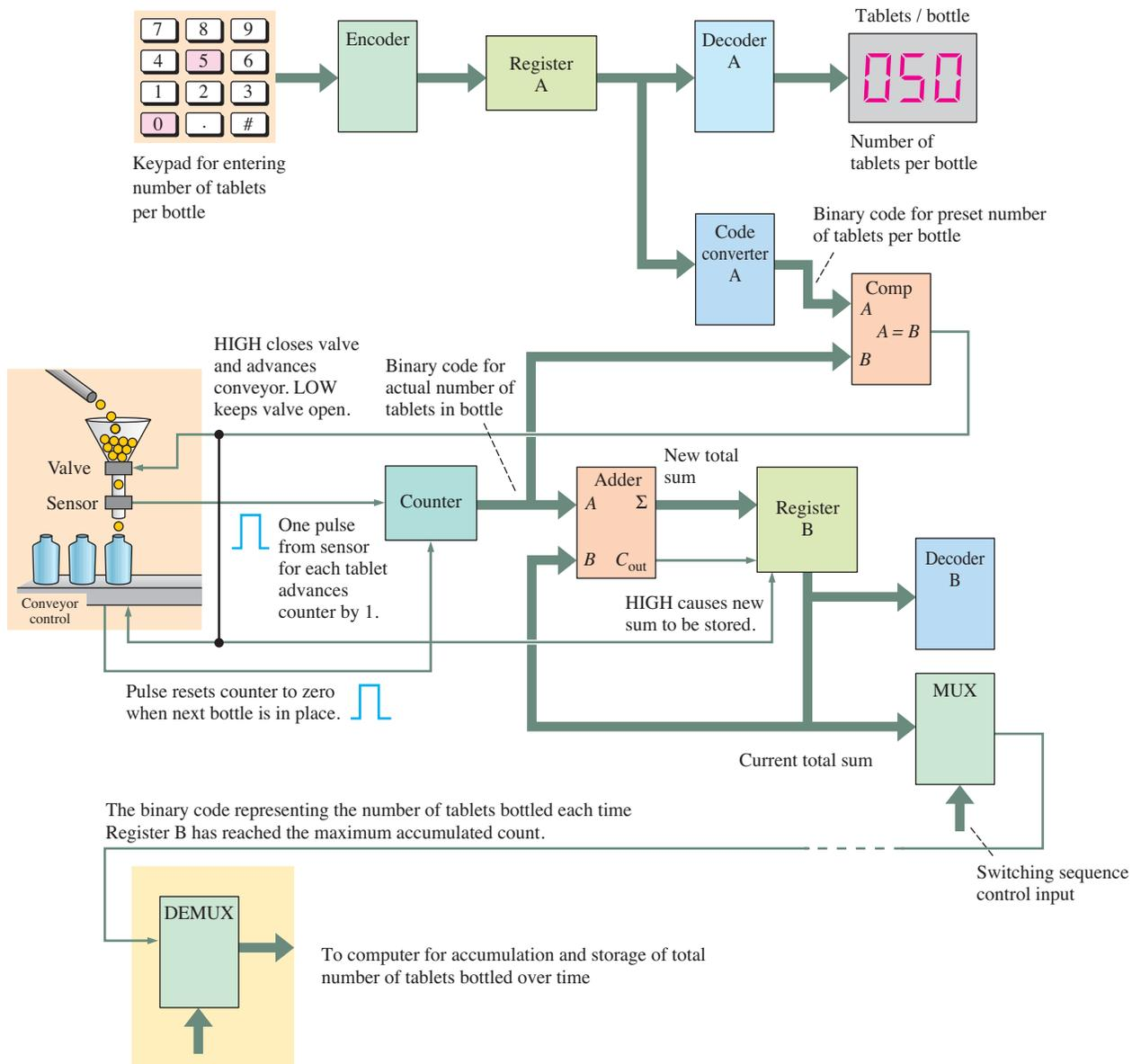
**FIGURE 1-28** Block diagram of a tablet-bottling system.
