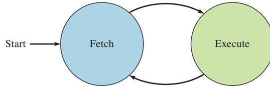
**FIGURE 14–11** The fetch/execute cycle of a processor.
