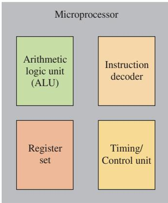
**FIGURE 14-9** Elements of a microprocessor (CPU).
