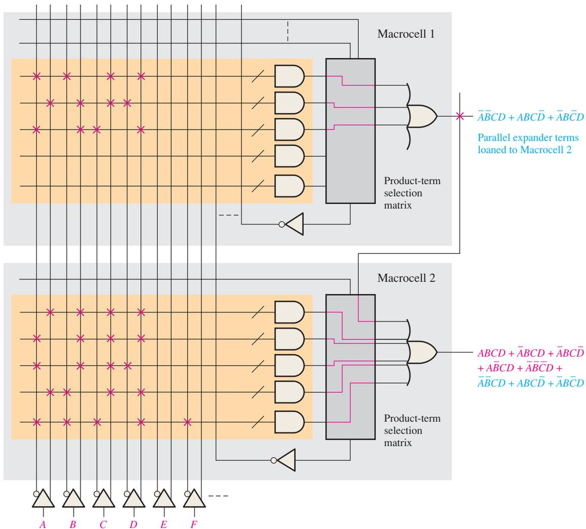
**FIGURE 10-14** Simplified illustration of using parallel expander terms from another macrocell to increase an SOP expression. The red Xs and lines represent the connections produced in the hardware by the software compiler running the programmed design.
