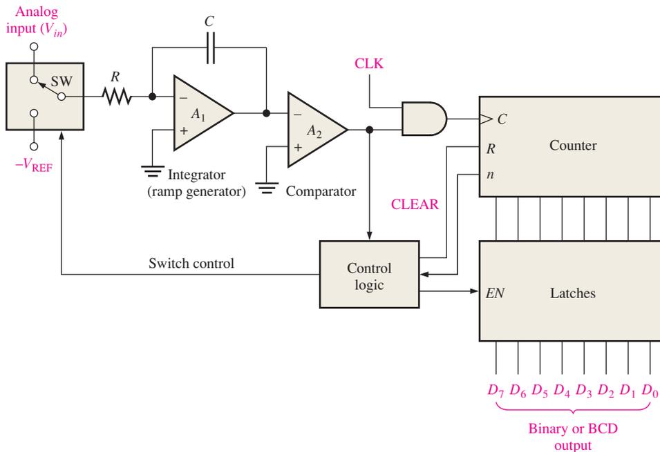
**FIGURE 12-15** Basic dual-slope ADC.
