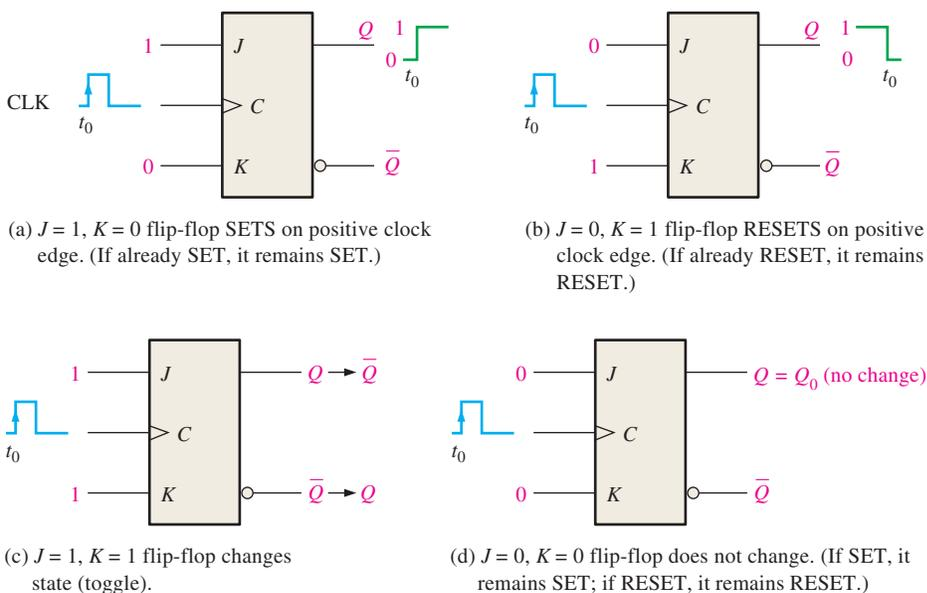
**FIGURE 7-17** Operation of a positive edge-triggered J-K flip-flop.
