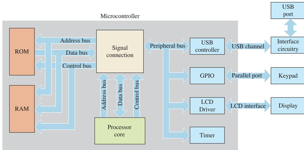
**FIGURE 14-35** Microcontroller block diagram for programmable calculator.
