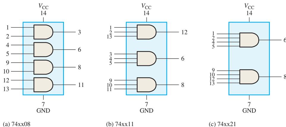
**FIGURE 3–59** 74 series AND gate devices with pin numbers.
