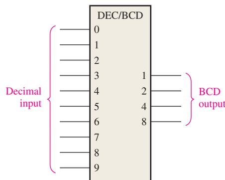
**FIGURE 6-36** Logic symbol for a decimal-to-BCD encoder.
