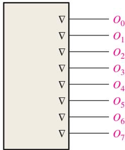
**FIGURE 13-77** Method of indicating tri-state outputs on an IC device.
