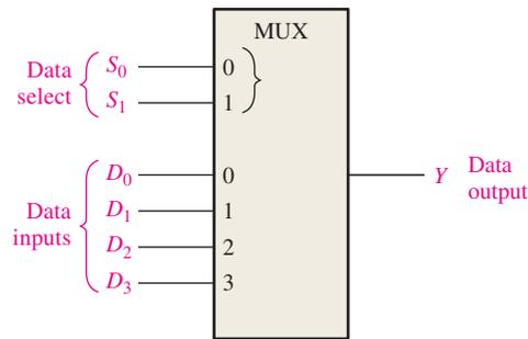
**FIGURE 6-43** Logic symbol for a 1-of-4 data selector/multiplexer.
