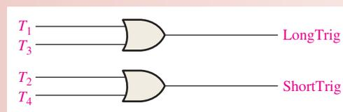
**FIGURE 6–68** Trigger logic.
