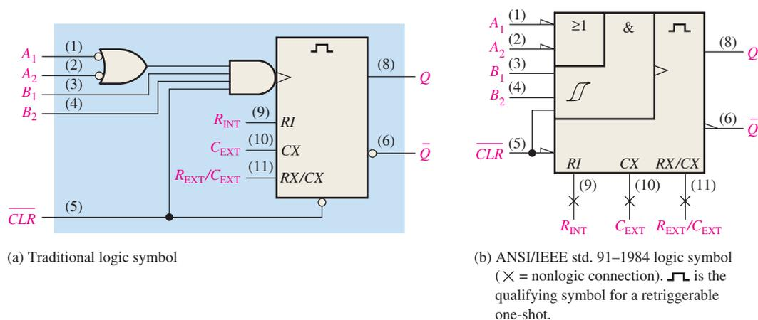
**FIGURE 7-49** Logic symbol for the 74LS122 retriggerable one-shot.
