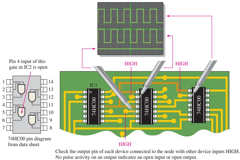
**FIGURE 5-46** Open input in a load device.
