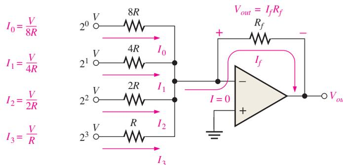
**FIGURE 12-26** A 4-bit DAC with binary-weighted inputs.
