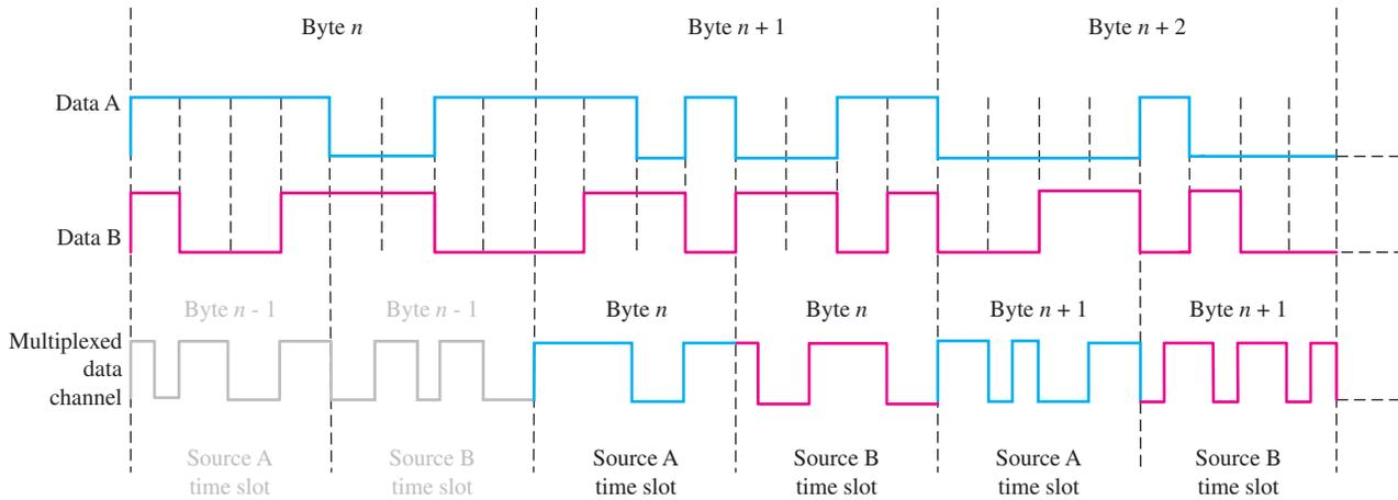
**FIGURE 13-44** Byte-interleaved TDM with two data sources.
