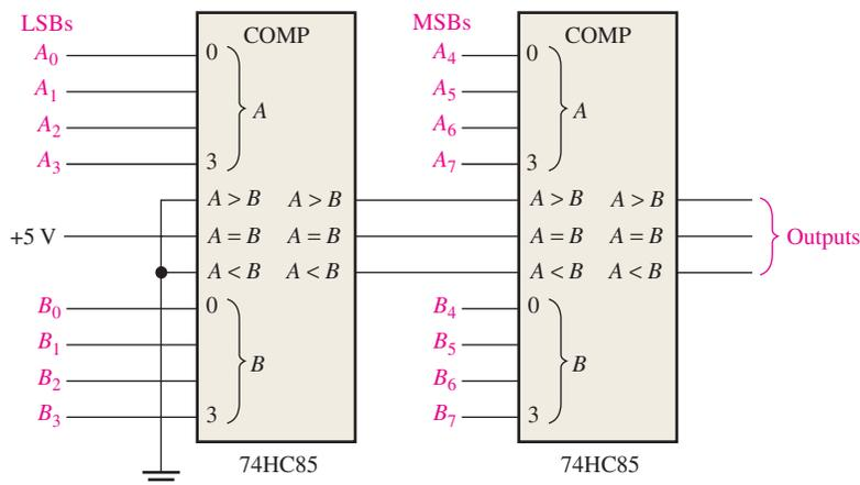
**FIGURE 6-25** An 8-bit magnitude comparator using two 74HC85s.
