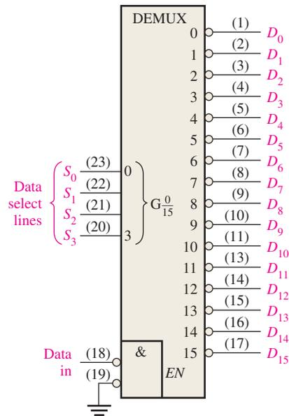
FIGURE 6-54 The decoder used as a demultiplexer.
