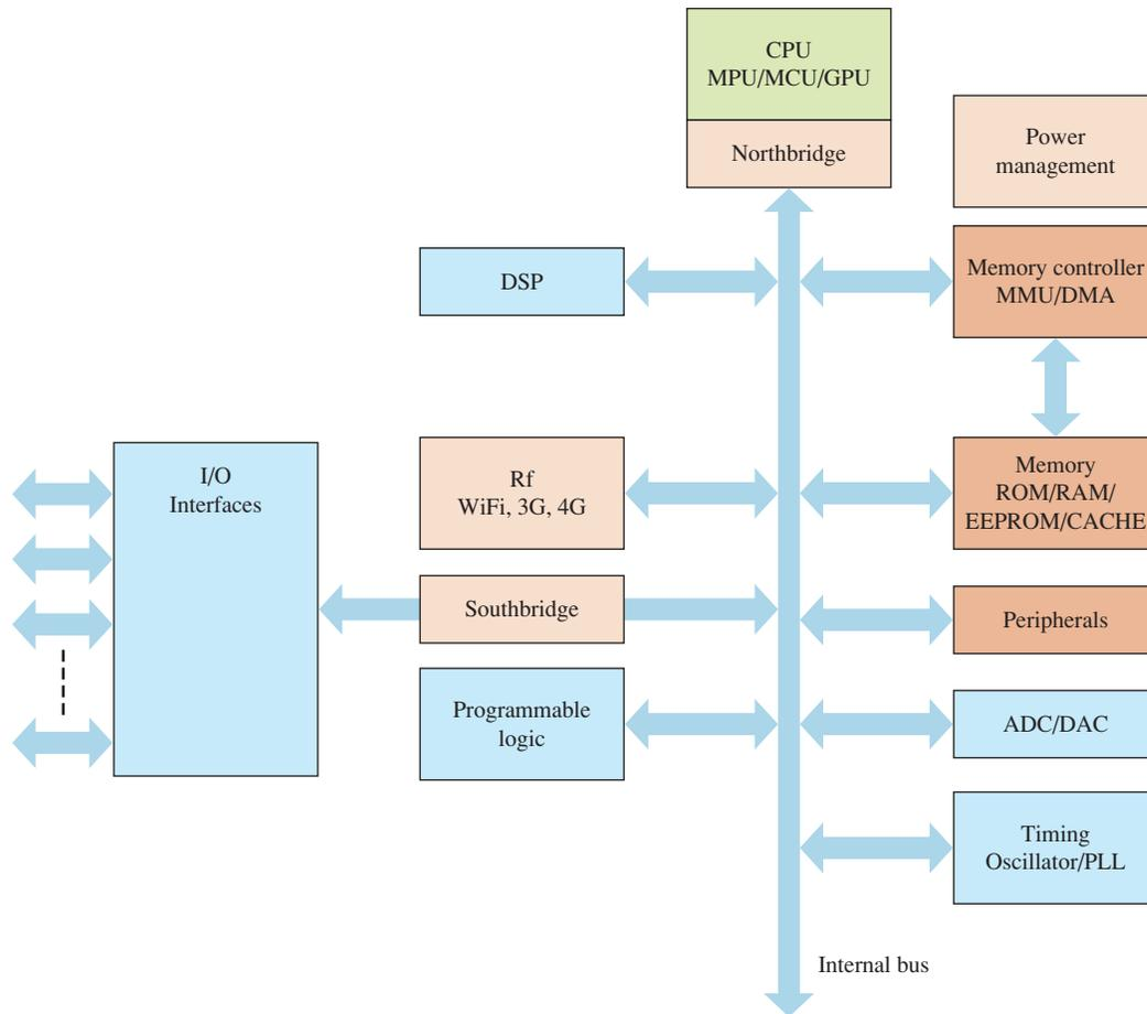
**FIGURE 14-38** Generic block diagram of a typical SoC.
