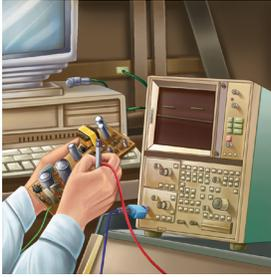
Troubleshooting is the process of recognizing, isolating, and correcting a fault or failure in a circuit or system. To be an effective troubleshooter, you must understand how the circuit or system is supposed to work and be able to recognize incorrect performance. For example, to determine whether or not a certain logic gate is faulty, you must know what the output should be for given inputs.
