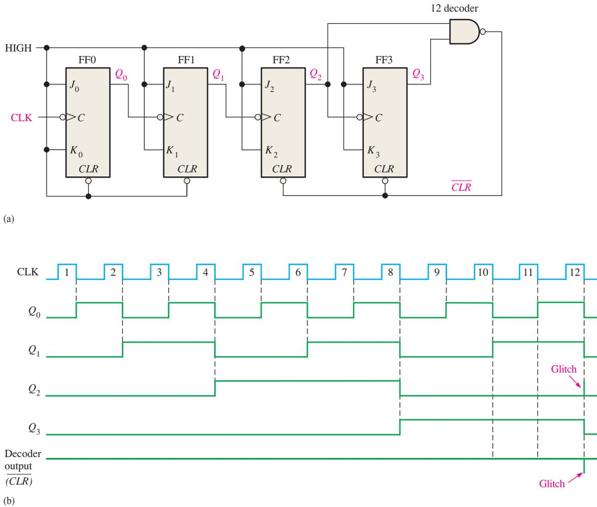
**FIGURE 9-10** Asynchronously clocked modulus-12 counter with asynchronous recycling.
