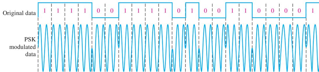
**FIGURE 13-22** Illustration of phase-shift keying (PSK).
