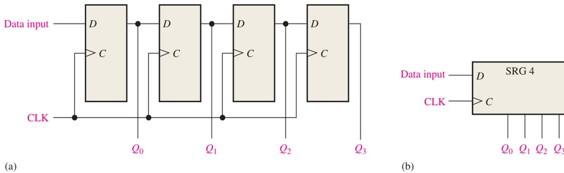
**FIGURE 8-6** A serial in/parallel out shift register.
