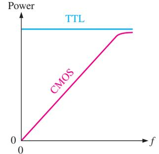
**FIGURE 15-7** Power-versus-frequency curves for TTL and CMOS.
