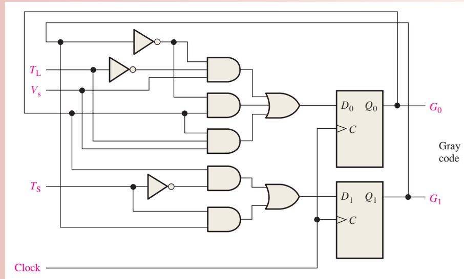
**FIGURE 7-69** Complete diagram for the sequential logic.
