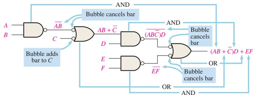
(b) Output expression can be obtained directly from the function of each gate symbol in the diagram.
