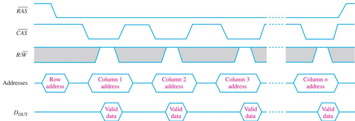
**FIGURE 11-22** Fast page mode timing for a read operation.
