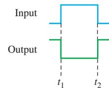
**FIGURE 3–3** Timing diagram for the case in Figure 3–2.
