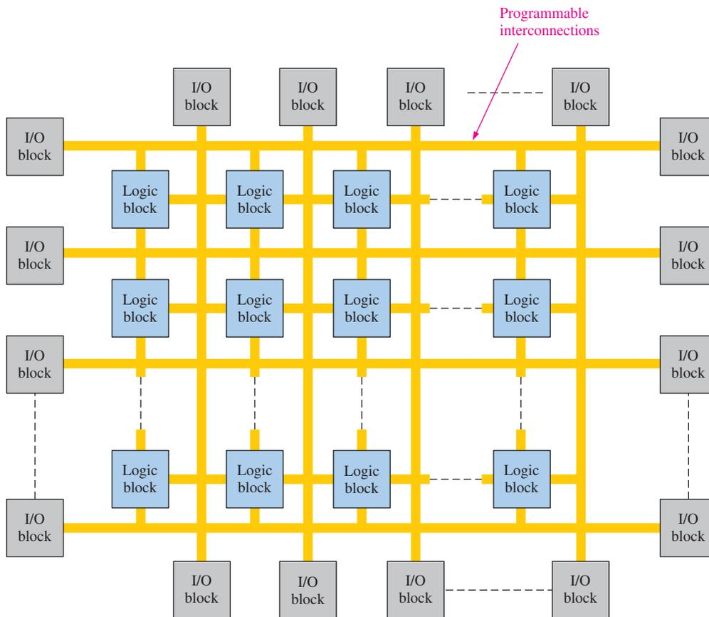
**FIGURE 1-34** Basic structure of an FPGA.
