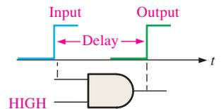
**FIGURE 15-8** A basic illustration of propagation delay time.
