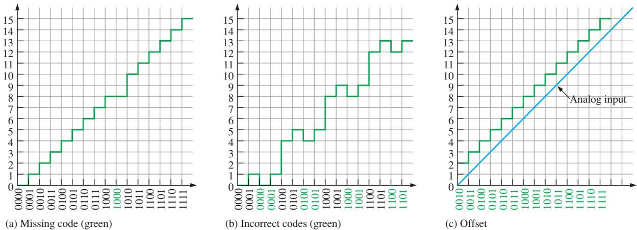
FIGURE 12-24 Illustrations of analog-to-digital conversion errors.
