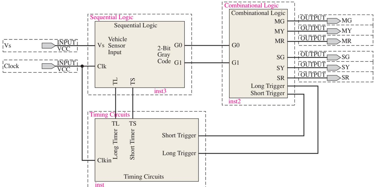
**FIGURE 10-36** Block diagram for the traffic signal controller.
