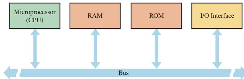
**FIGURE 13-74** The interconnection of microprocessor-based system components by a bidirectional, multiplexed bus.
