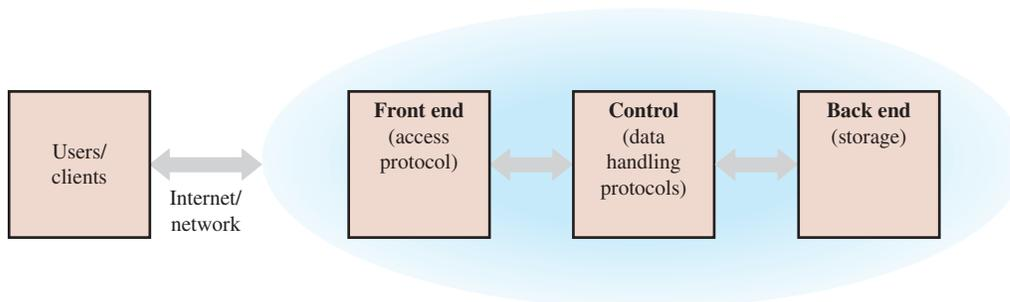
**FIGURE 11-71** Generic architecture of a cloud storage system.
