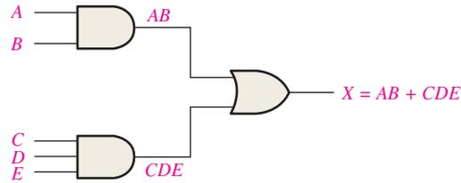
**FIGURE 5-9** Logic circuit for  $X = AB + CDE$ .
