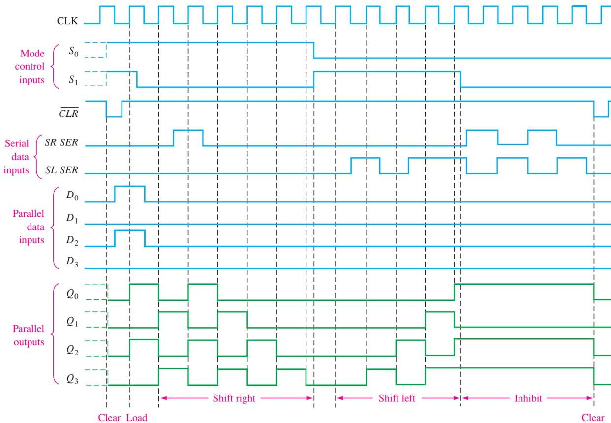
**FIGURE 8-20** Sample timing diagram for a 74HC194 shift register.
