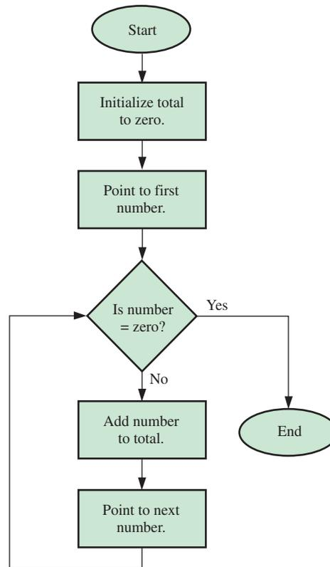
**FIGURE 14–32** Flowchart for adding a list of numbers.
