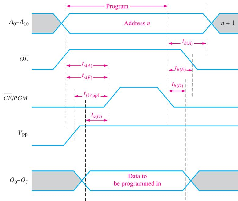
**FIGURE 11-32** Timing diagram for a  $2048 \times 8$  EPROM programming cycle, with critical setup times ( $t_s$ ) and hold times ( $t_h$ ) indicated.
