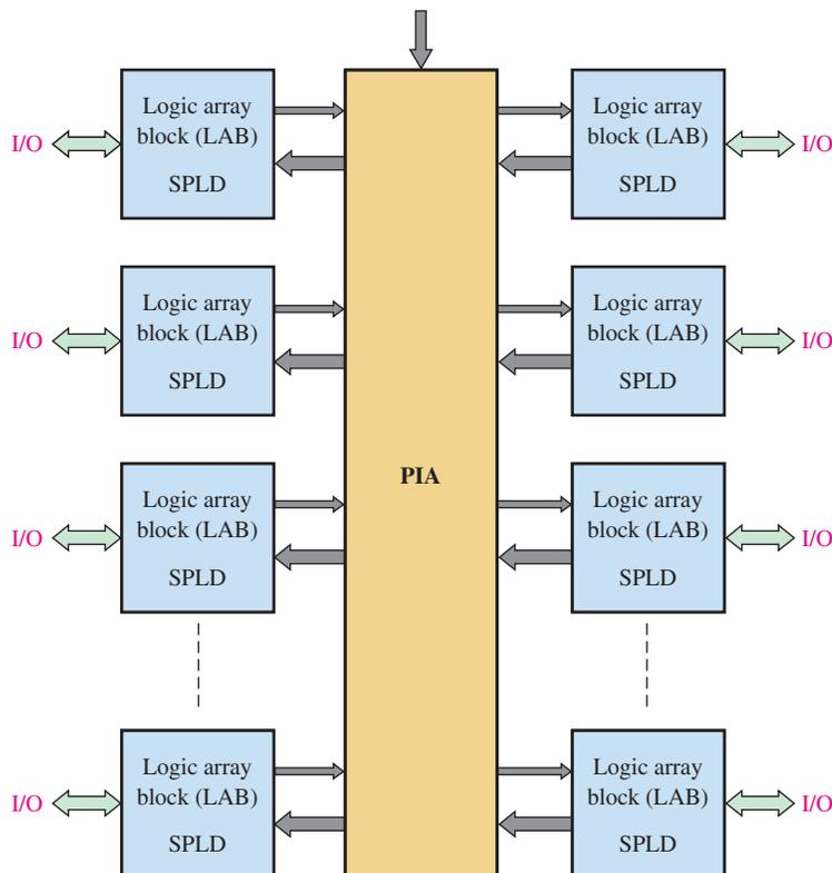
**FIGURE 10-8** Basic block diagram of a generic CPLD.
