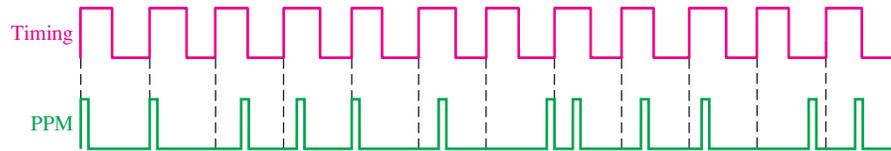
**FIGURE 13-33** Example of a PPM signal with timing.
