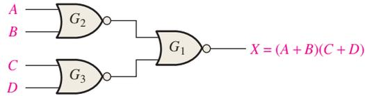
**FIGURE 5-26** NOR logic for  $X = (A + B)(C + D)$ .
