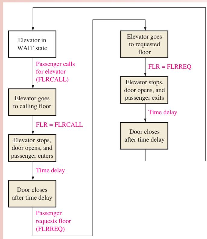
**FIGURE 9–60** One cycle of the elevator operation.
