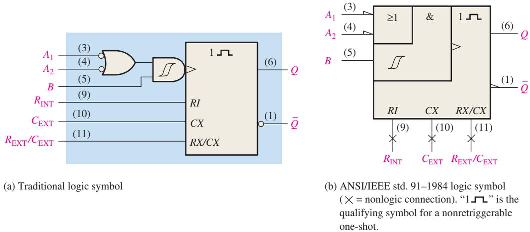
**FIGURE 7-47** Logic symbols for the 74121 nonretriggerable one-shot.
