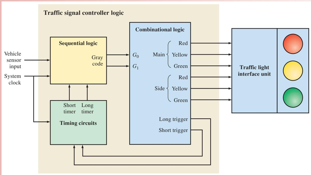
**FIGURE 6-64** Block diagram of the traffic signal controller.
