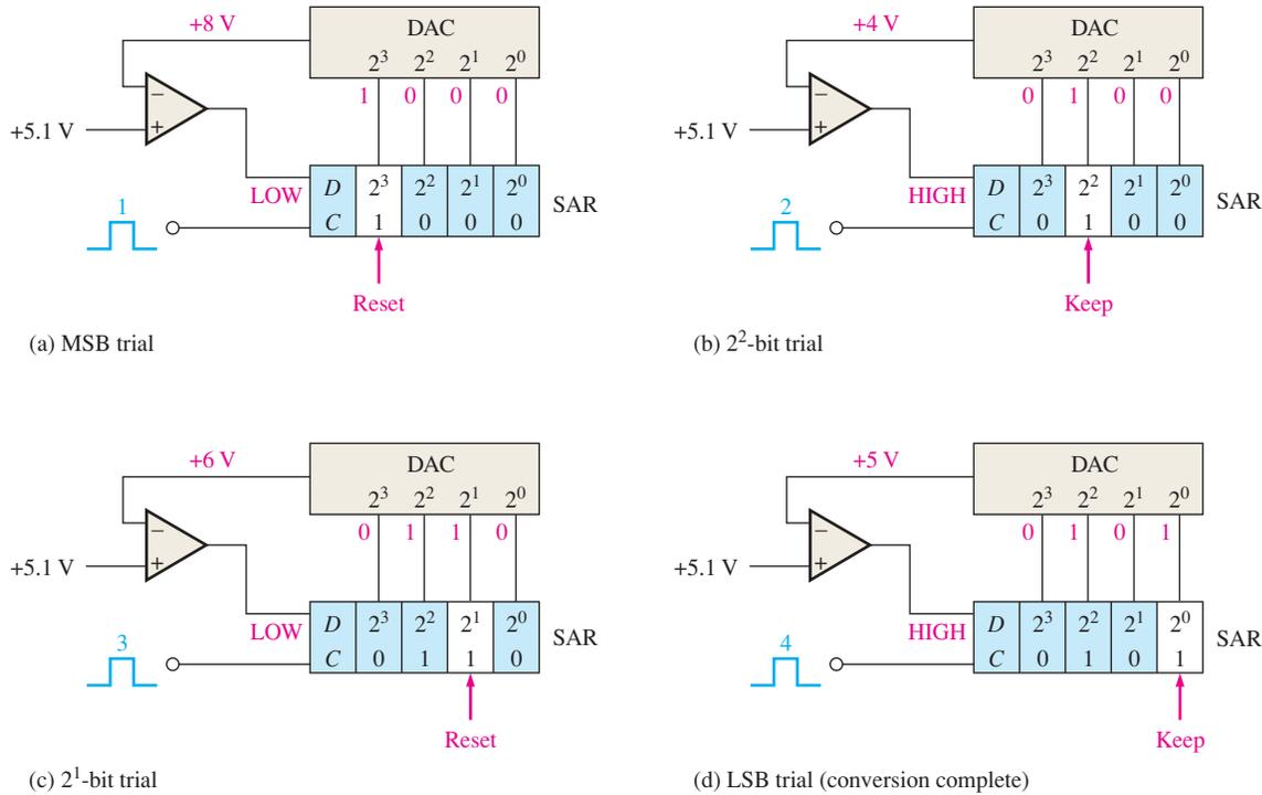
**FIGURE 12-18** Illustration of the successive-approximation conversion process.
