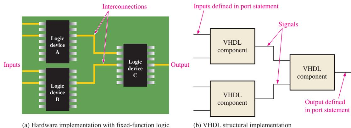
**FIGURE 5–37** Simplified comparison of the VHDL structural approach to a hardware implementation. The VHDL signals correspond to the interconnections on the circuit board, and the VHDL components correspond to the 74 series IC devices.
