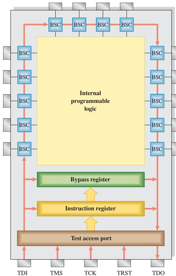
**FIGURE 10-45** Greatly simplified diagram of a JTAG compliant (IEEE Std. 1149.1) programmable logic device (CPLD or FPGA). The BSCs (boundary scan cells) form the boundary scan register. Only a small number of BSCs are shown for illustration.
