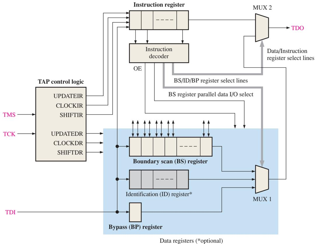
**FIGURE 10–46** Boundary scan logic diagram.
