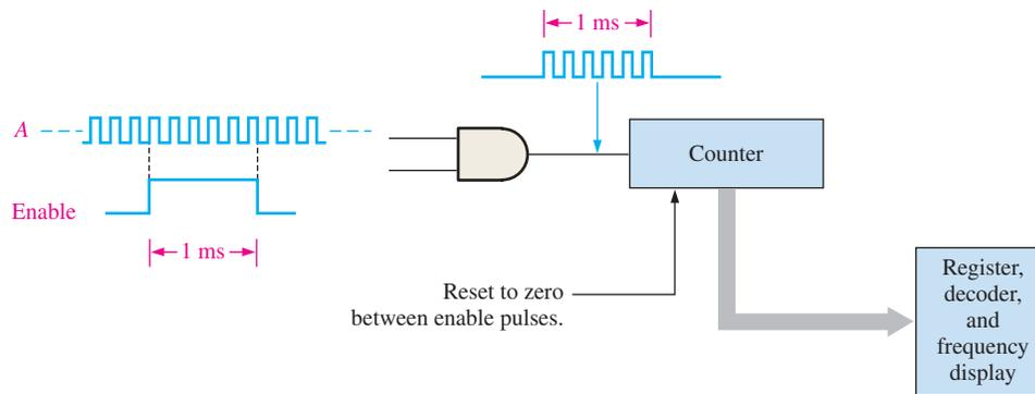
**FIGURE 3-16** An AND gate performing an enable/inhibit function for a frequency counter.
