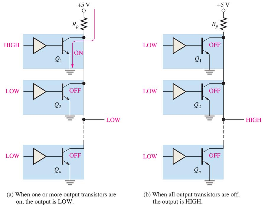
**FIGURE 15-38** Open-collector wired negative-AND operation with inverters.
