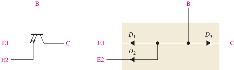
FIGURE 15-30 Diode equivalent of a TTL multiple-emitter transistor.
