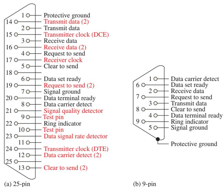
**FIGURE 13-68** Standard RS-232 connectors.
