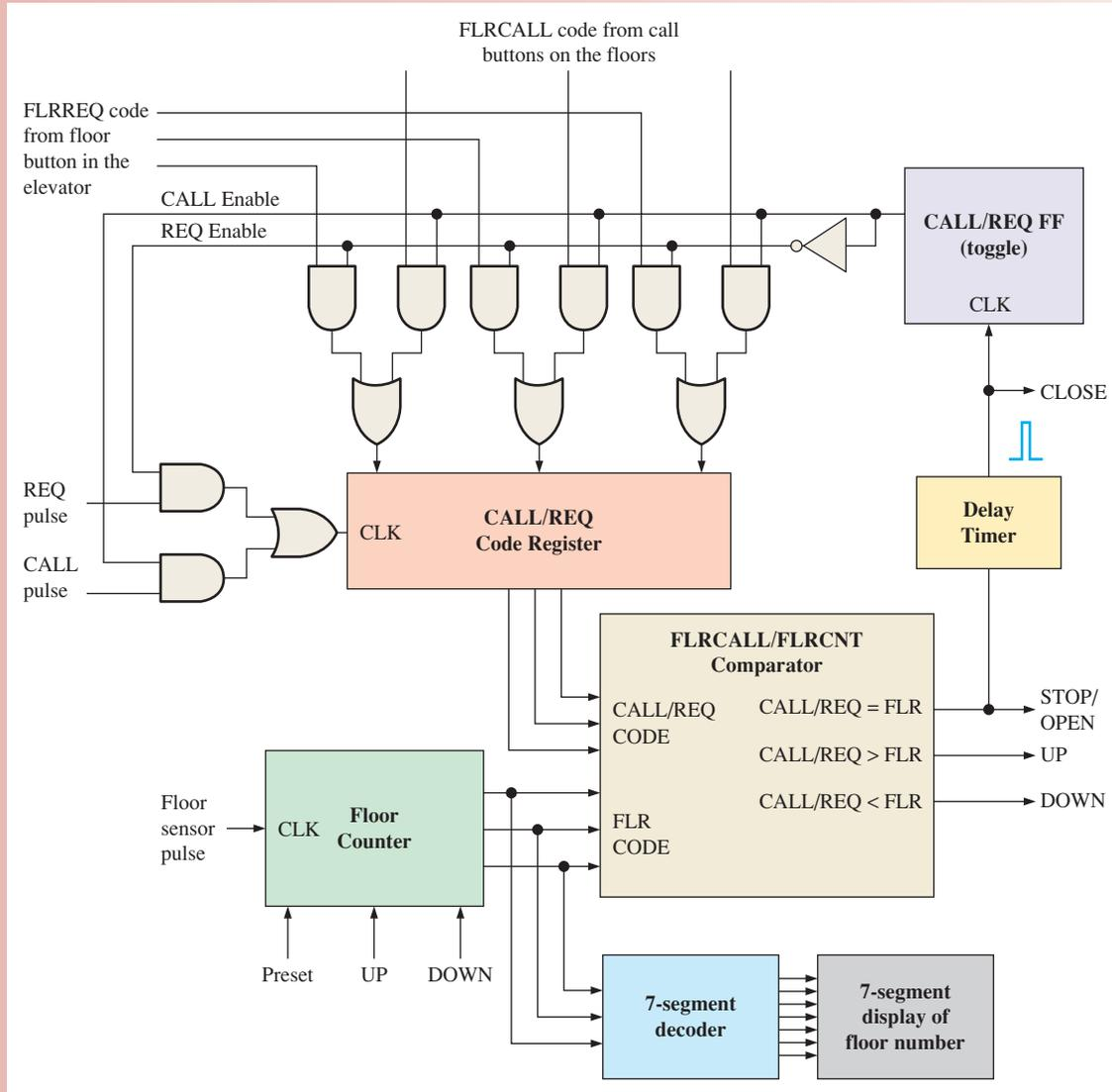
**FIGURE 9–64** Elevator controller logic diagram.
