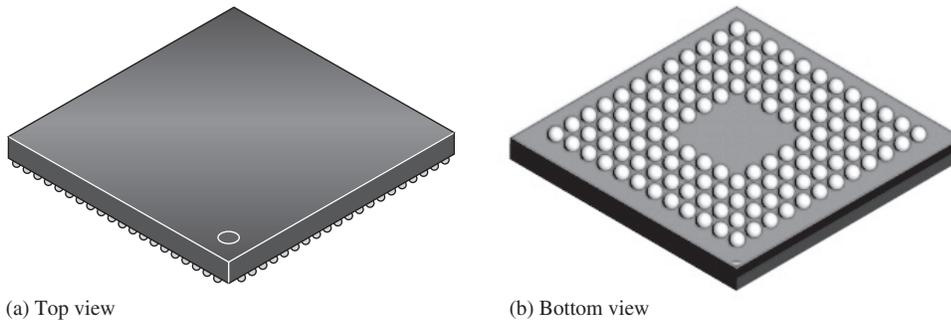
**FIGURE 1-35** A typical ball-grid array (BGA) package.
