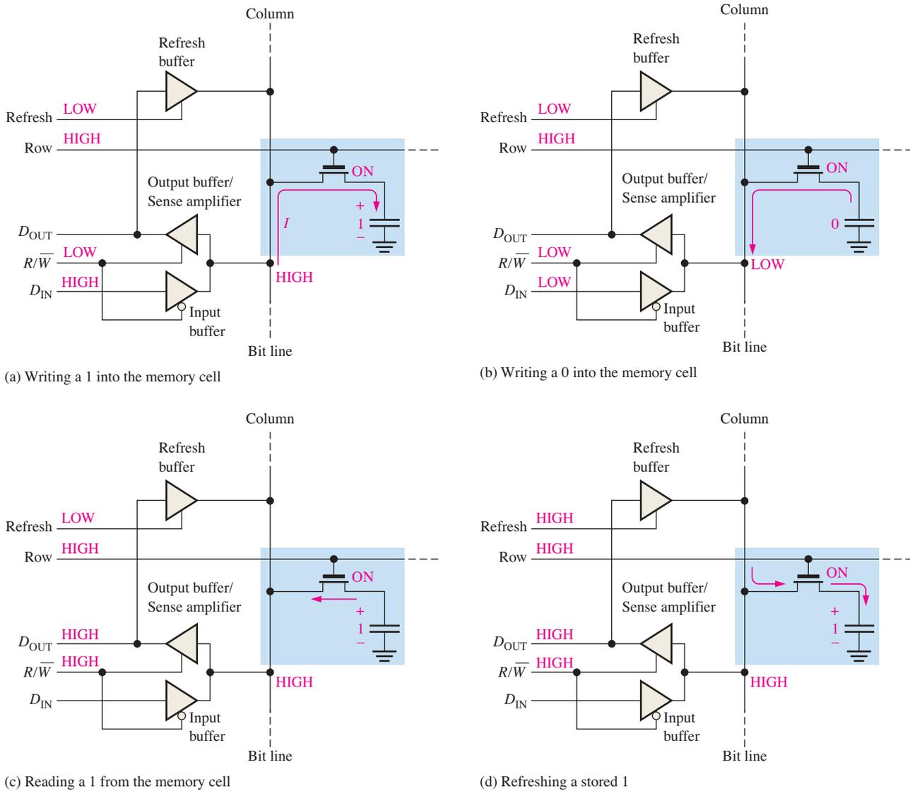
**FIGURE 11-18** Basic operation of a DRAM cell.
