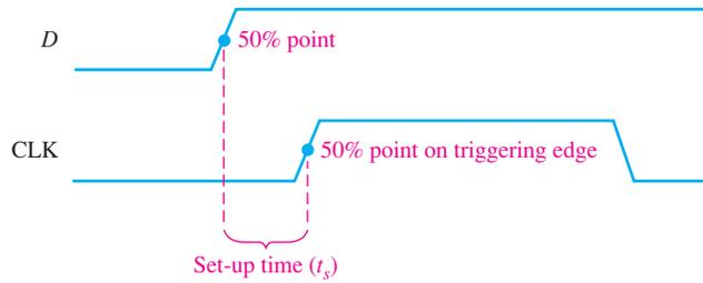
**FIGURE 7-33** Set-up time ( $t_s$ ). The logic level must be present on the  $D$  input for a time equal to or greater than  $t_s$  before the triggering edge of the clock pulse for reliable data entry.
