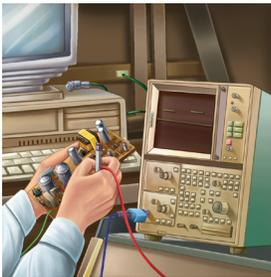
A traditional method of troubleshooting sequential logic and other more complex systems uses a procedure of “exercising” the circuit under test with a known input waveform (stimulus) and then observing the output for the correct bit pattern.
