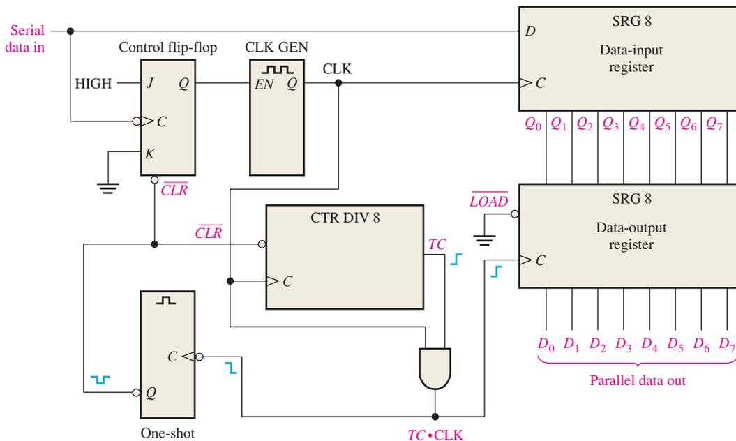
**FIGURE 8–31** Simplified logic diagram of a serial-to-parallel converter.
