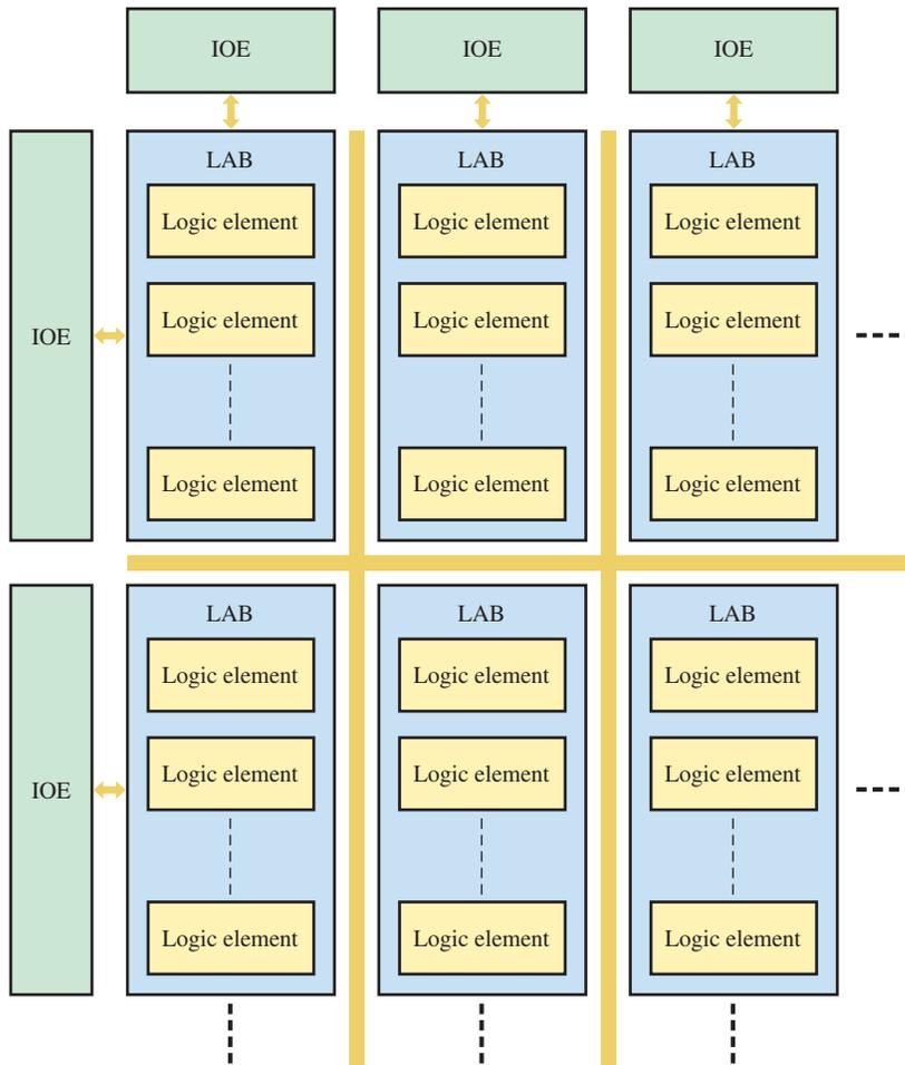
**FIGURE 10-15** Simplified block diagram of an LUT CPLD.
