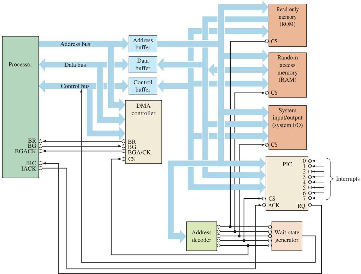
**FIGURE 14-25** Block diagram of a typical computer.
