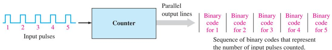
**FIGURE 1–27** Illustration of basic counter operation.
