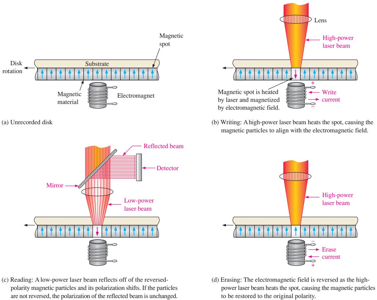
**FIGURE 11–63** Basic principle of a magneto-optical disk.
