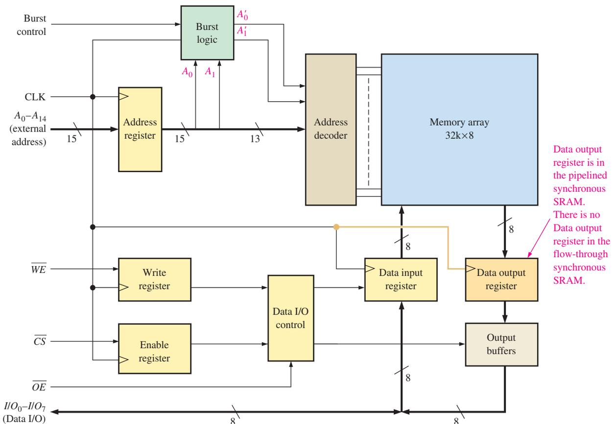
**FIGURE 11–14** A basic block diagram of a synchronous SRAM with burst feature.
