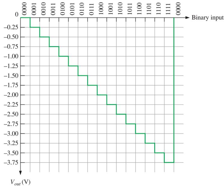
**FIGURE 12-28** Output of the DAC in Figure 12-27.
