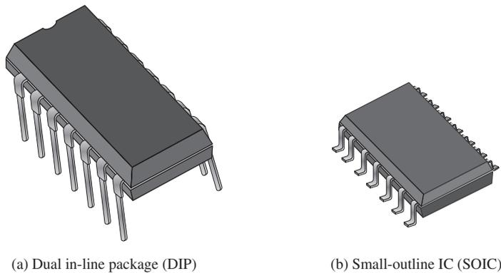
**FIGURE 1-39** Examples of through-hole and surface-mounted devices. The DIP is larger than the SOIC with the same number of leads. This particular DIP is approximately 0.785 in. long, and the SOIC is approximately 0.385 in. long.
