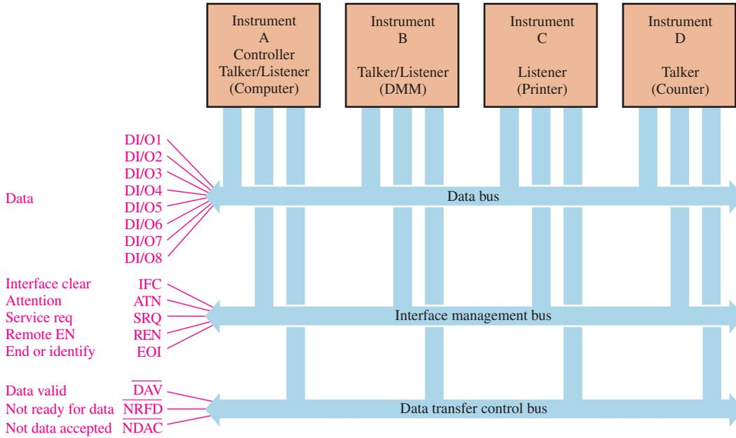
**FIGURE 13-58** A typical IEEE 488 (GPIB) connection.
