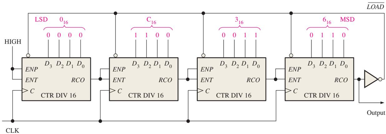
**FIGURE 9–41** A divide-by-40,000 counter using 74HC161 4-bit binary counters. Note that each of the parallel data inputs is shown in binary order (the right-most bit  $D_0$  is the LSB in each counter).
