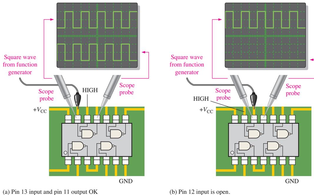
**FIGURE 3-70** Troubleshooting a NAND gate for an open input.
