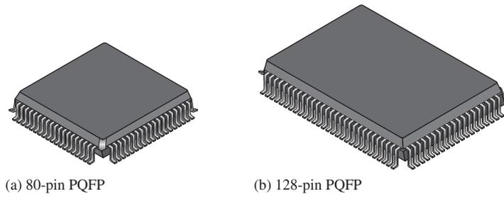
**FIGURE 1-33** Typical CPLD plastic quad flat packages (PQFP).
