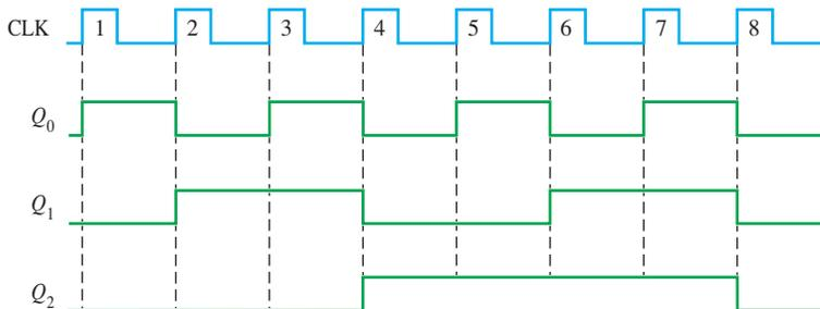
**FIGURE 9–16** Timing diagram for the counter of Figure 9–15.
