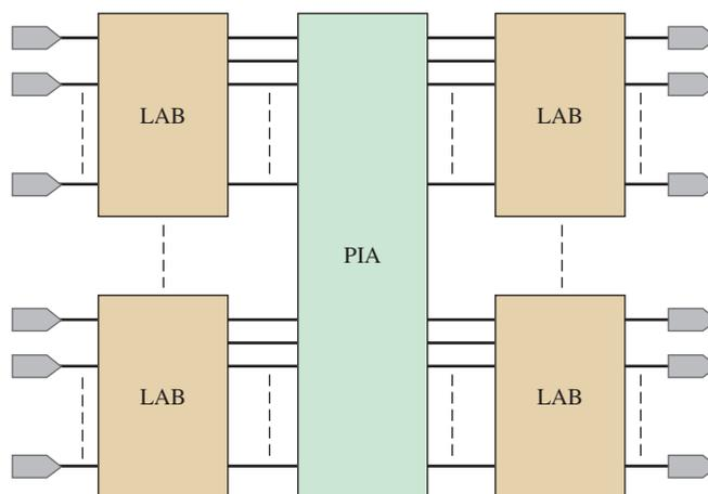
**FIGURE 1-32** General block diagram of a CPLD.
