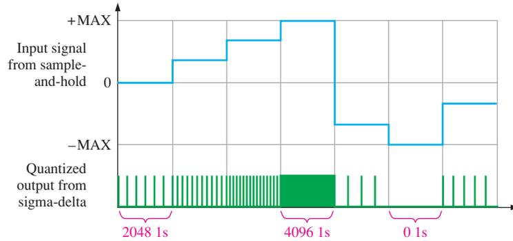
**FIGURE 12-20** A simplified illustration of sigma-delta analog-to-digital conversion.
