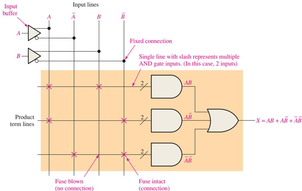
**FIGURE 10–4** A portion of a programmed PAL/GAL.
