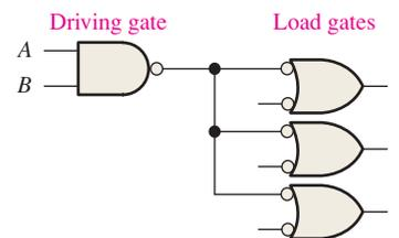
**FIGURE 15-10** Loading a gate output with gate inputs.
