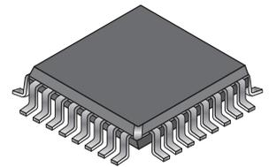
**FIGURE 1-31** A typical SPLD package.
