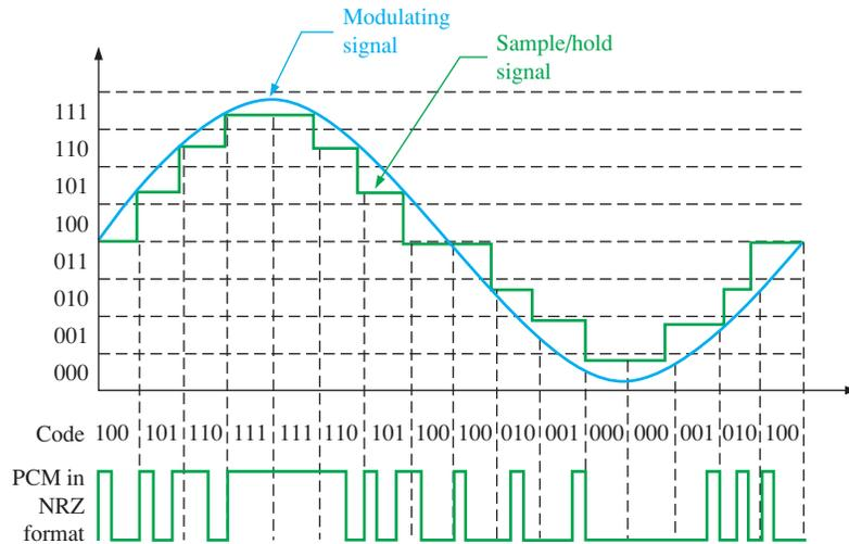
**FIGURE 13-37** Concept of PCM with eight levels.
