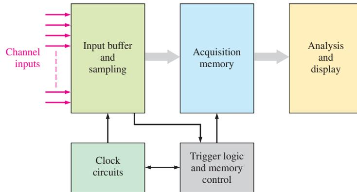
**FIGURE 1-51** Simplified block diagram of a logic analyzer.
