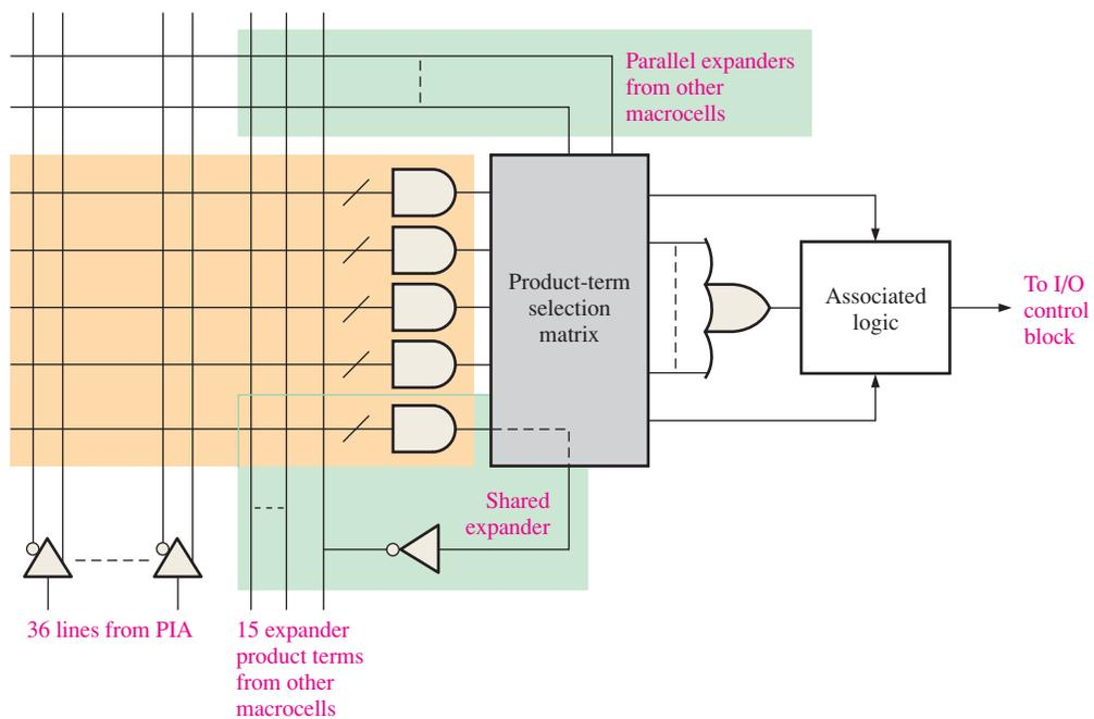
**FIGURE 10-10** Simplified diagram of a macrocell in a typical CPLD.
