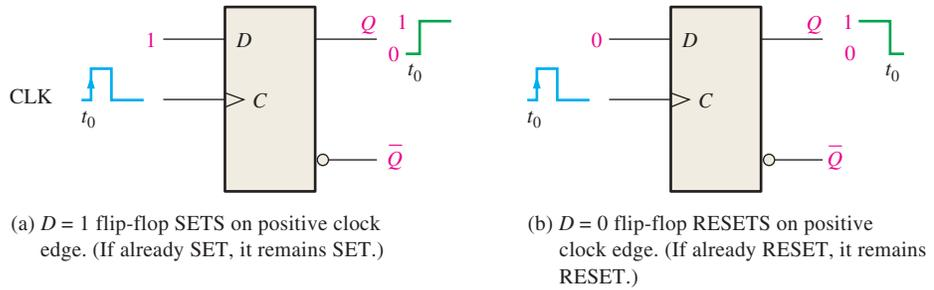
**FIGURE 7-14** Operation of a positive edge-triggered D flip-flop.
