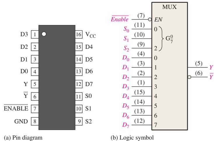
**FIGURE 6–47** The 74HC151 eight-input data selector/multiplexer.
