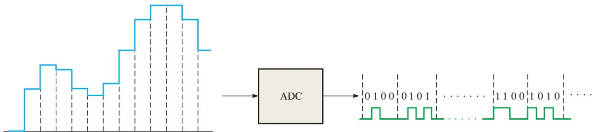
**FIGURE 12-6** Basic function of an analog-to-digital converter (ADC) (The binary codes and number of bits are arbitrarily chosen for illustration only). The ADC output waveform that represents the binary codes is also shown.
