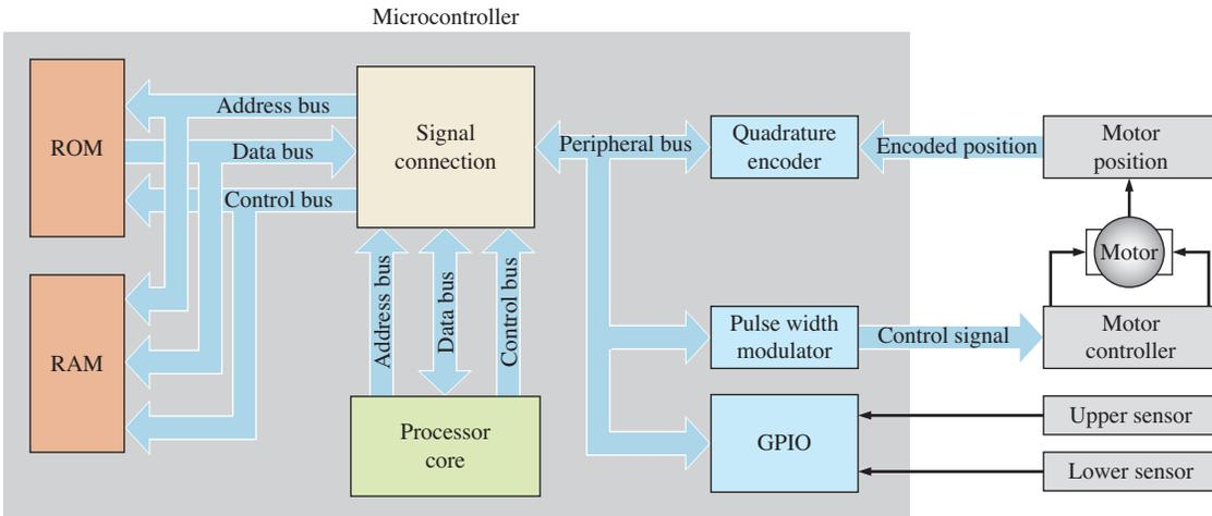
**FIGURE 14-36** Basic block diagram for a robotics system.
