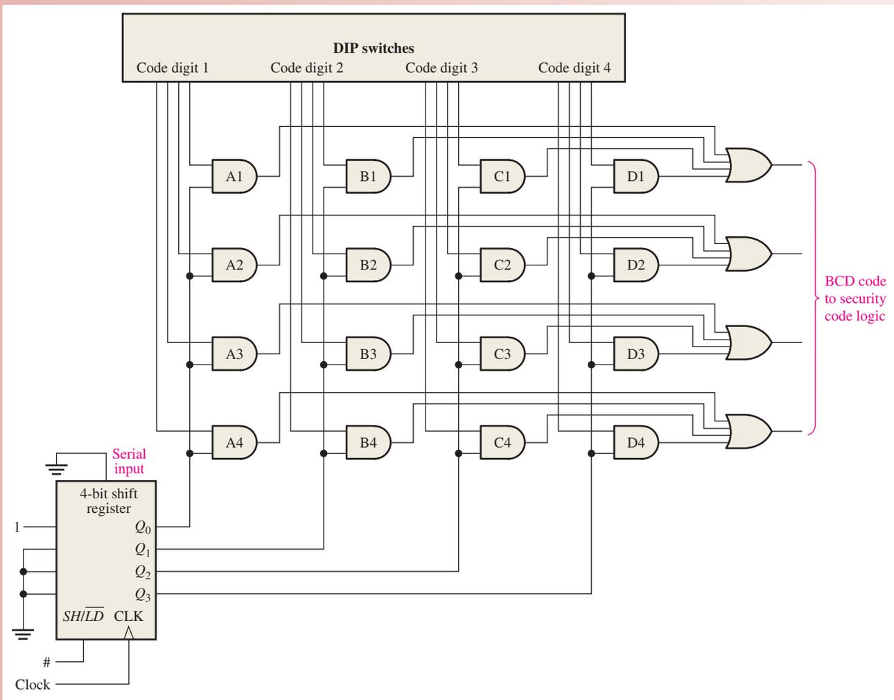
**FIGURE 8–44** Logic diagram of the code-selection logic.
