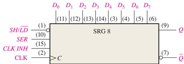
**FIGURE 8-12** The 74HC165 8-bit parallel load shift register.
