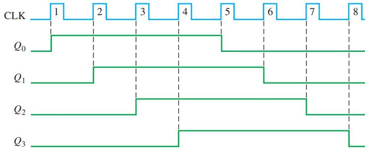
**FIGURE 8-22** Timing sequence for a 4-bit Johnson counter.
