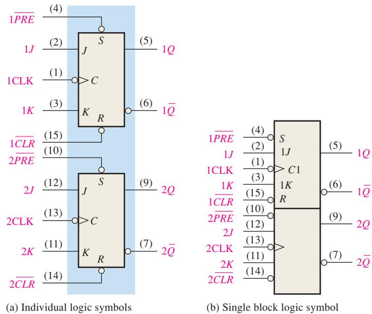
**FIGURE 7-29** The 74HC112 dual negative edge-triggered J-K flip-flop.
