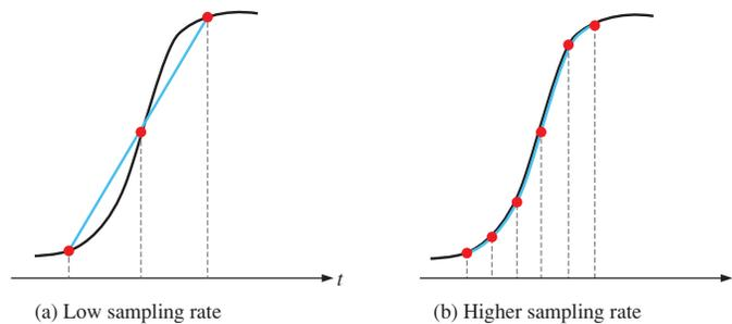
**FIGURE 1–49** Example of sampling a waveform. The dashed lines represent the clock (sampling) rate. The incoming signal is black and the resulting representation is blue. The red dots are the points at which the waveform values are sampled.
