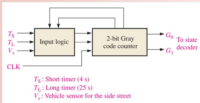
FIGURE 7-67 Block diagram of the sequential logic.
