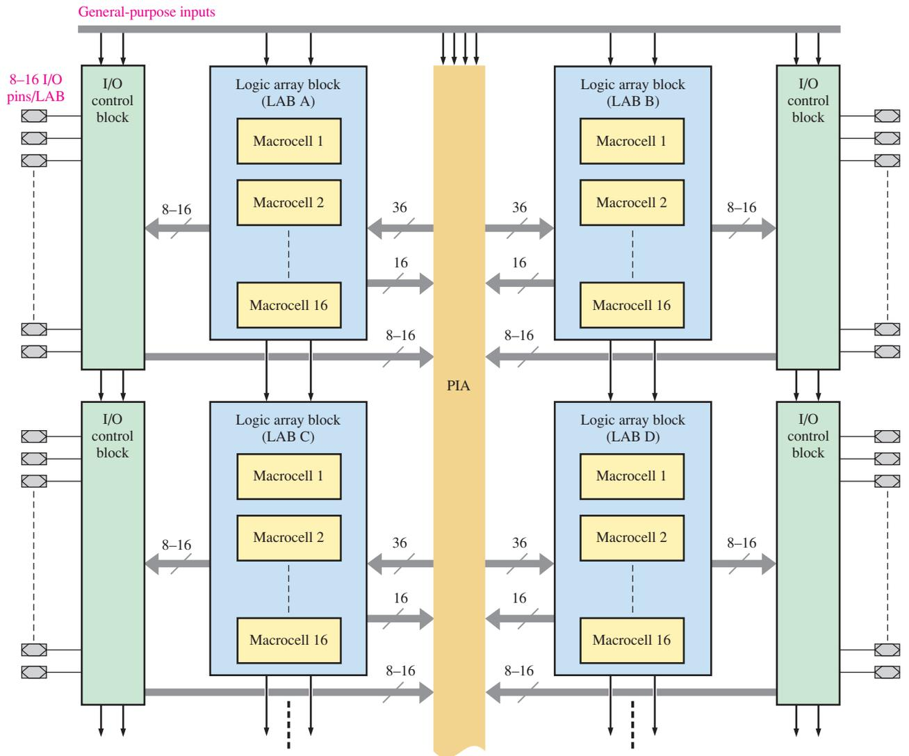
**FIGURE 10-9** Basic block diagram of a typical CPLD.
