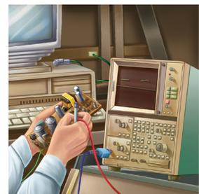
is known to be correct. One way of doing this is illustrated in Figure 11–72. This process requires a reference ROM that contains the same data as the ROM to be tested. A special test instrument is programmed to read each address in both ROMs simultaneously and to compare the contents. A flowchart in Figure 11–73 illustrates the basic sequence.
