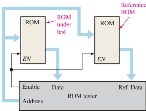
**FIGURE 11-72** Block diagram for a complete contents check of a ROM.
