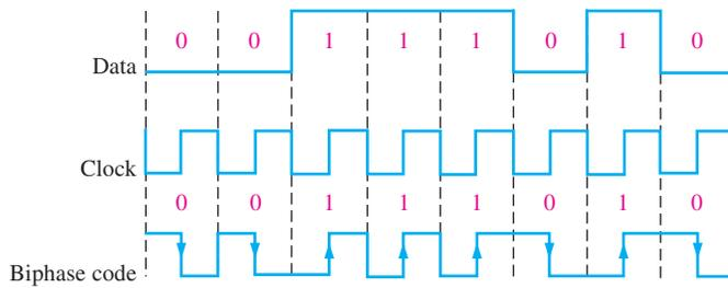
**FIGURE 13-16** Example of Manchester encoded data and timing.
