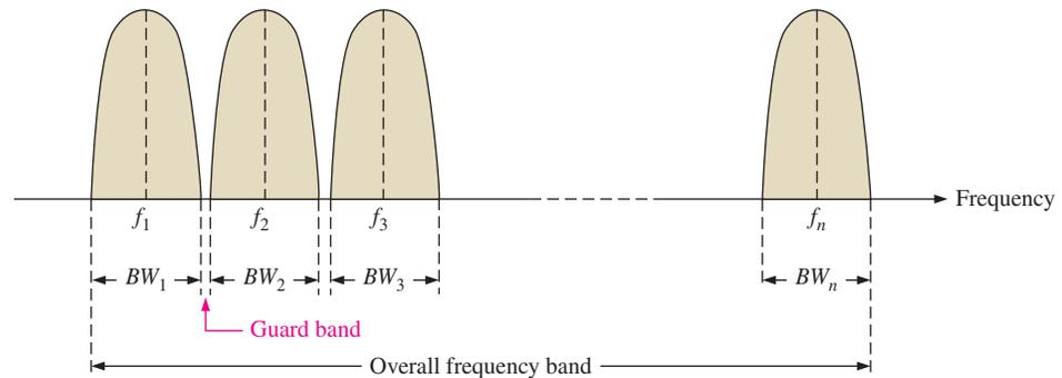
**FIGURE 13–49** Frequency spectrum of an FDM transmission.
