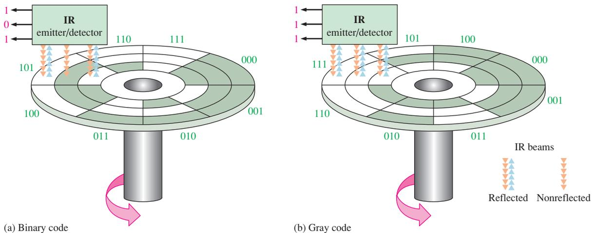
**FIGURE 2-7** A simplified illustration of how the Gray code solves the error problem in shaft position encoders. Three bits are shown to illustrate the concept, although most shaft encoders use more than 10 bits to achieve a higher resolution.
