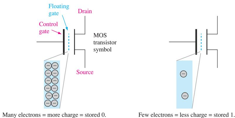
**FIGURE 11-33** The storage cell in a flash memory.
