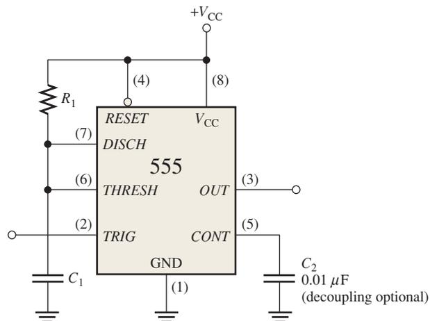
**FIGURE 7-53** The 555 timer connected as a one-shot.
