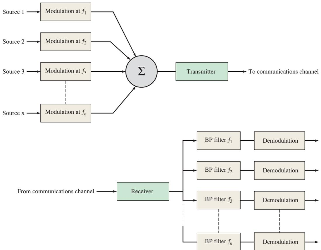
**FIGURE 13–48** Basic FDM system. Σ stands for summation.
