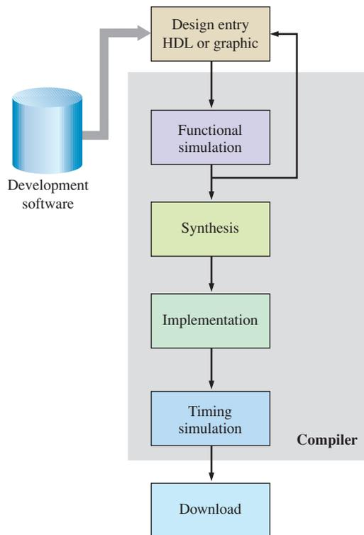
**FIGURE 1-37** Basic programmable logic design flow block diagram.
