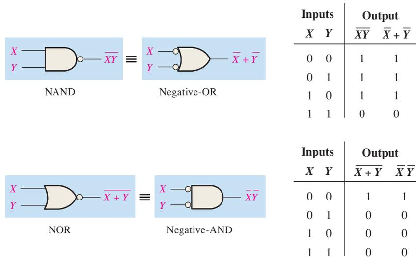
**FIGURE 4-17** Gate equivalencies and the corresponding truth tables that illustrate DeMorgan’s theorems. Notice the equality of the two output columns in each table. This shows that the equivalent gates perform the same logic function.
