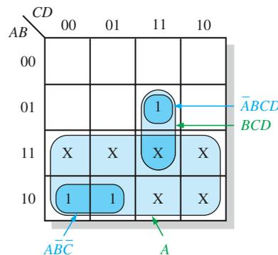
(b) Without “don’t cares”  $Y = \bar{A}\bar{B}\bar{C} + \bar{A}\bar{B}C\bar{D}$
