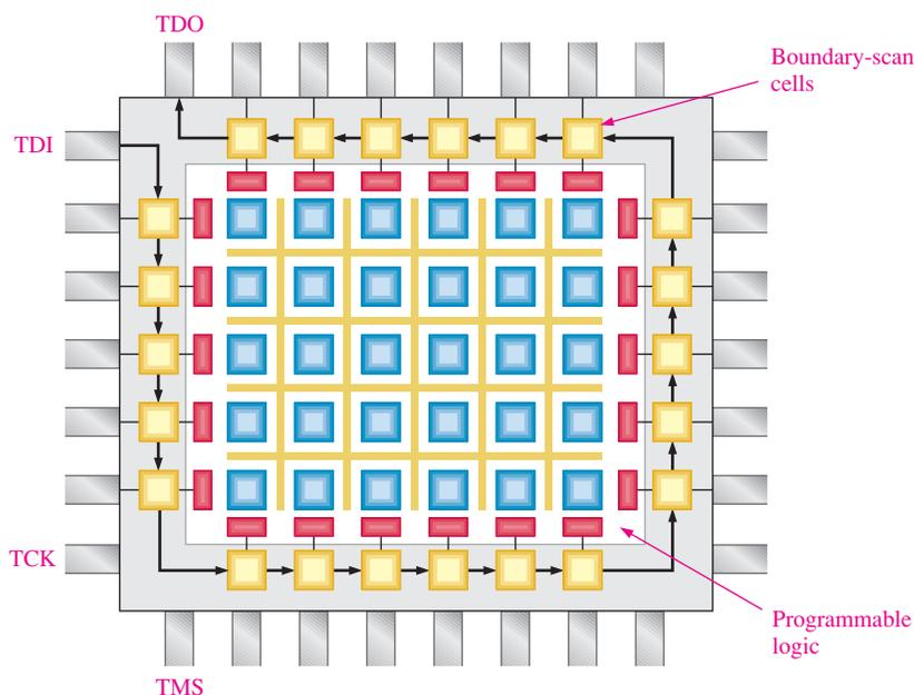
FIGURE 10-59 Basic concept of boundary scan logic in a programmable logic device.
