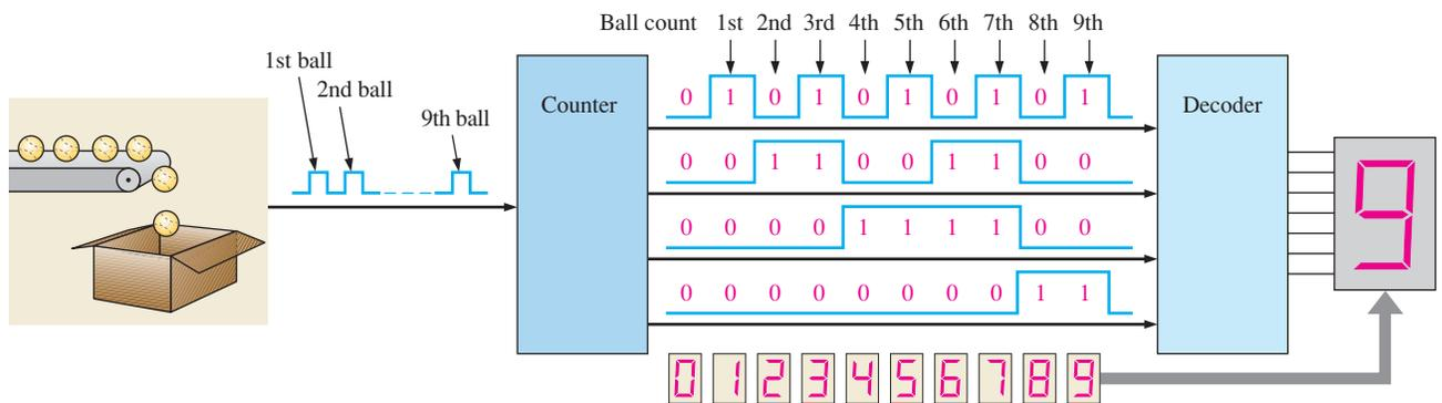
**FIGURE 2-1** Illustration of a simple binary counting application.
