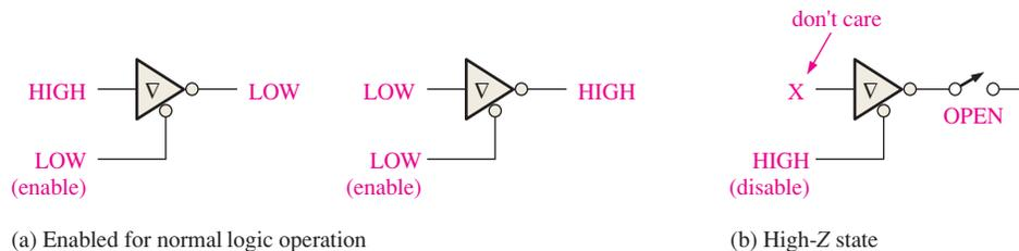
**FIGURE 15-22** The three states of a tri-state circuit.
