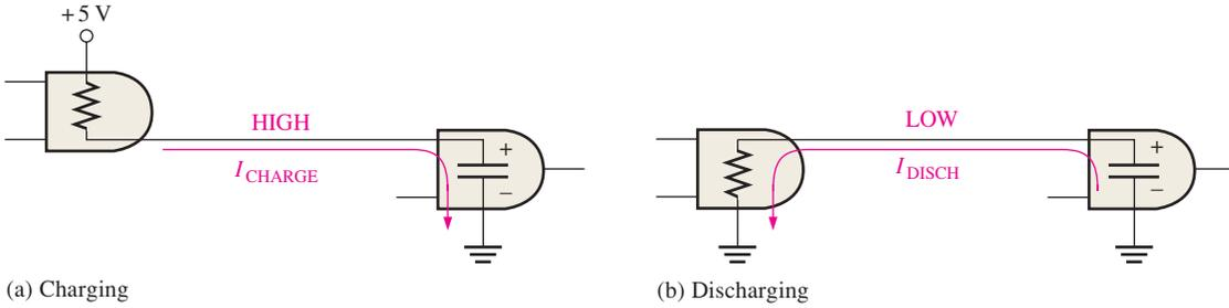
**FIGURE 15-11** Capacitive loading of a CMOS gate.
