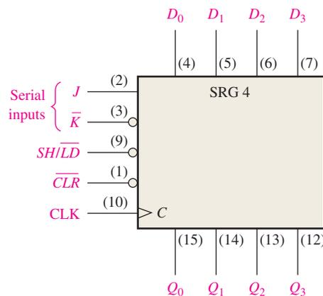
**FIGURE 8-15** The 74HC195 4-bit parallel access shift register.
