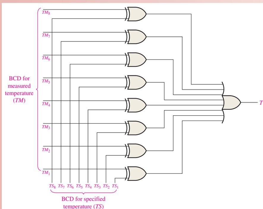
**FIGURE 5–52** Logic diagram of the temperature control logic.
