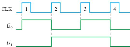
**FIGURE 9–14** Timing diagram for the counters of Figure 9–12.
