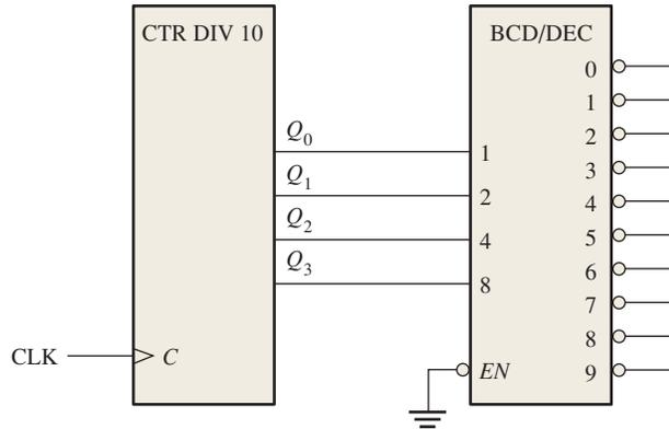
**FIGURE 9-44** A basic decade (BCD) counter and decoder.
