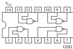
FIGURE 3-66 Bipolar logic. Partial data sheet for a 54/74LS00 quad 2-input NAND gate.
