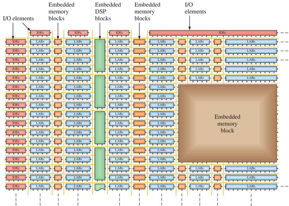
**FIGURE 10-33** Example FPGA block diagram.
