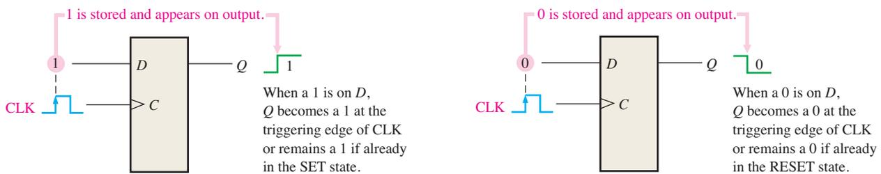
**FIGURE 8-1** The flip-flop as a storage element.
