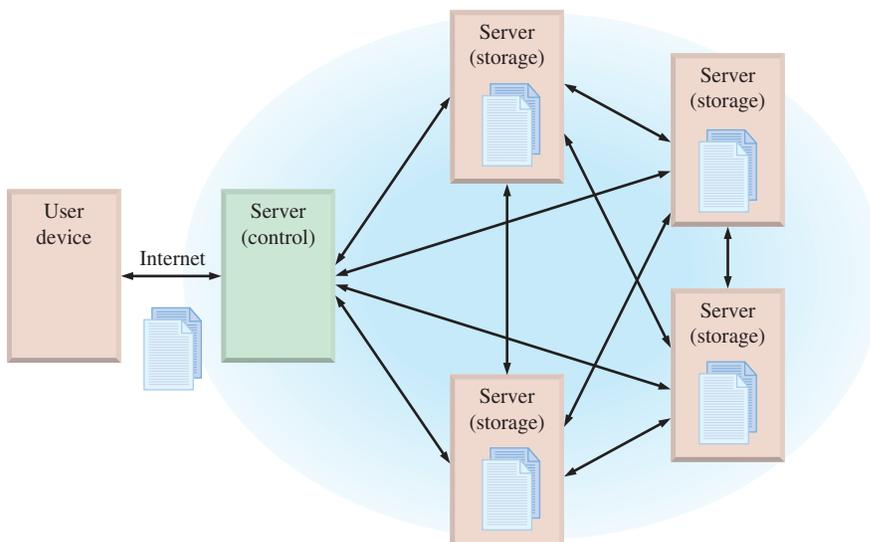
**FIGURE 11-70** A simple cloud storage system with storage redundancy. In this case, the data are stored on four different servers.
