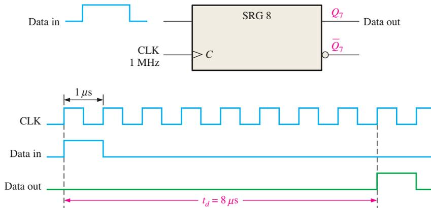
**FIGURE 8-26** The shift register as a time-delay device.
