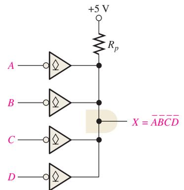
**FIGURE 15-37** A wired-AND configuration of four inverters.
