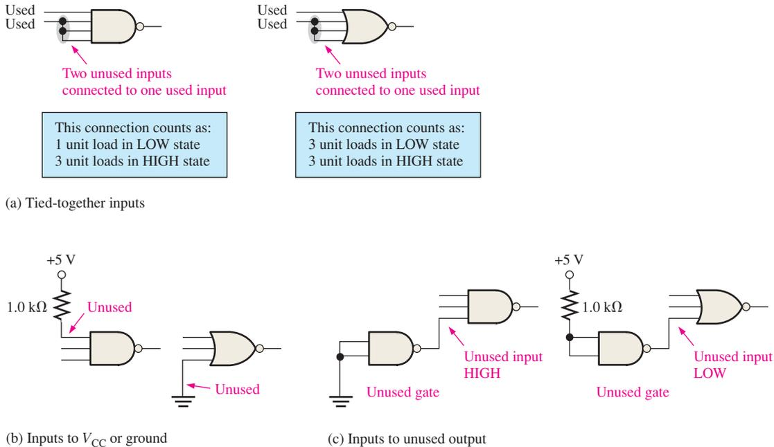
**FIGURE 15-45** Methods for handling unused TTL inputs.
