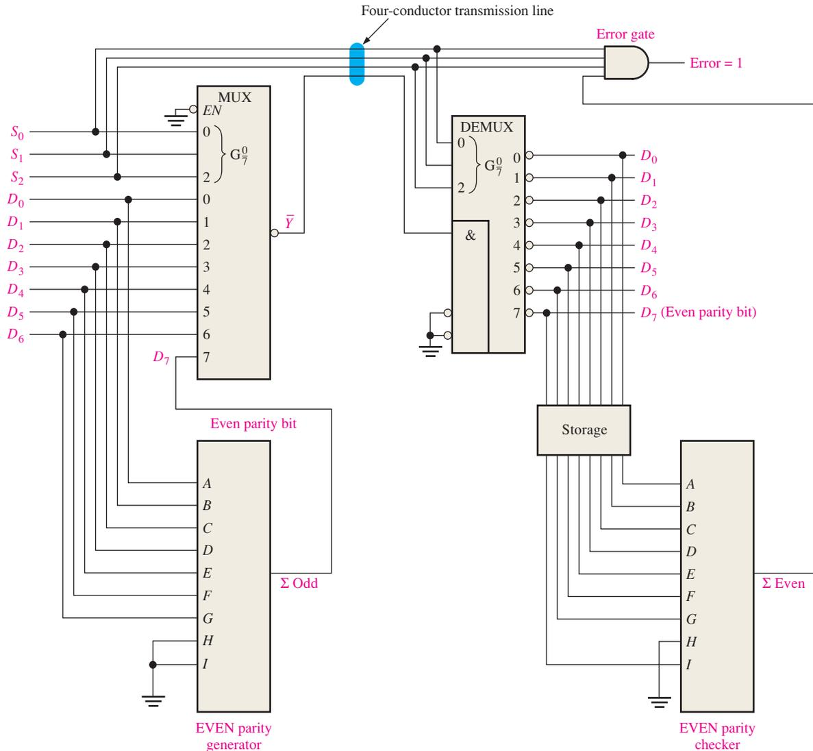
**FIGURE 6-58** Simplified data transmission system with error detection.
