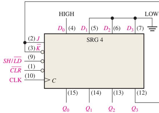
**FIGURE 8–29** 74HC195 connected as a ring counter.
