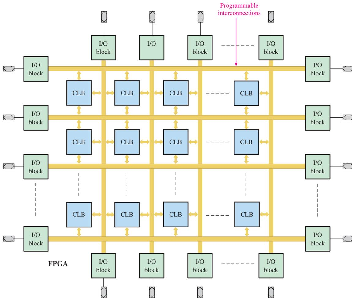
**FIGURE 10-23** Basic structure of an FPGA. CLB is configurable logic block, also known as logic array block (LAB).
