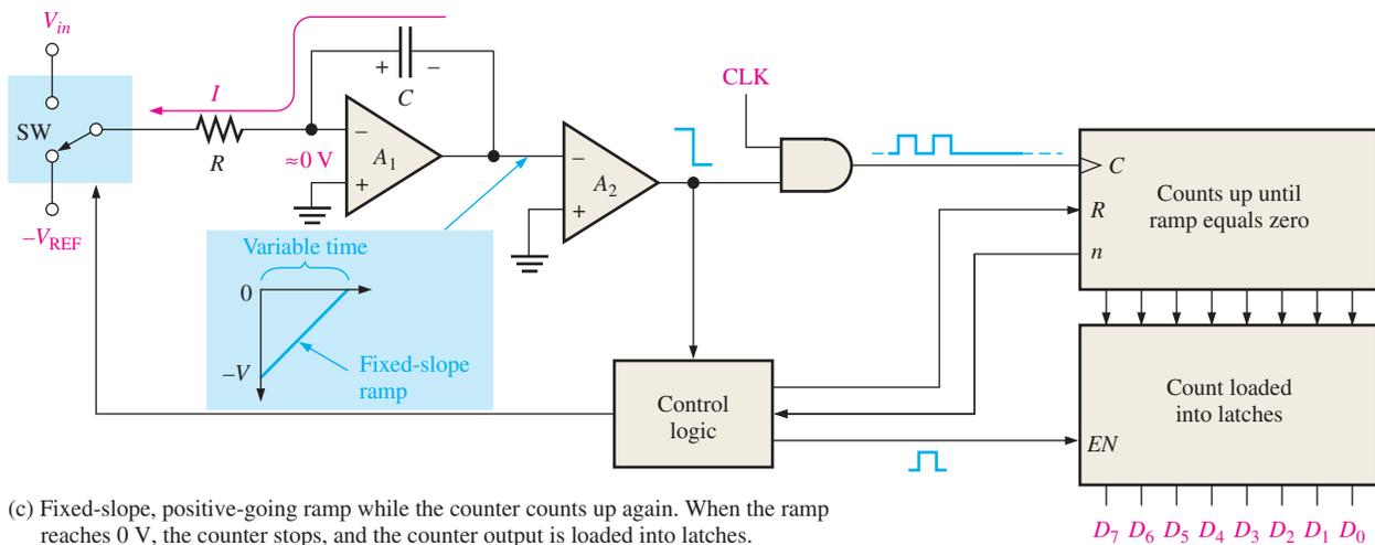
(c) Fixed-slope, positive-going ramp while the counter counts up again. When the ramp reaches 0 V, the counter stops, and the counter output is loaded into latches.
