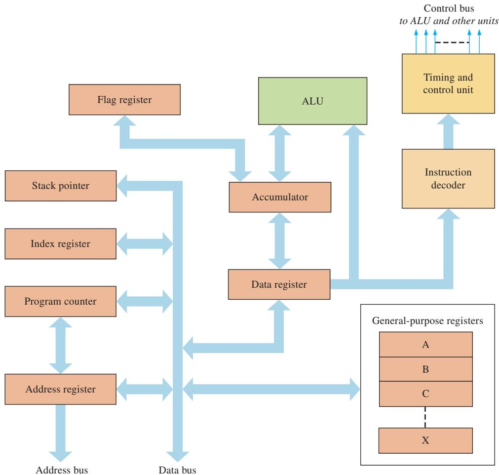
**FIGURE 14-10** Basic model of a simplified processor.
