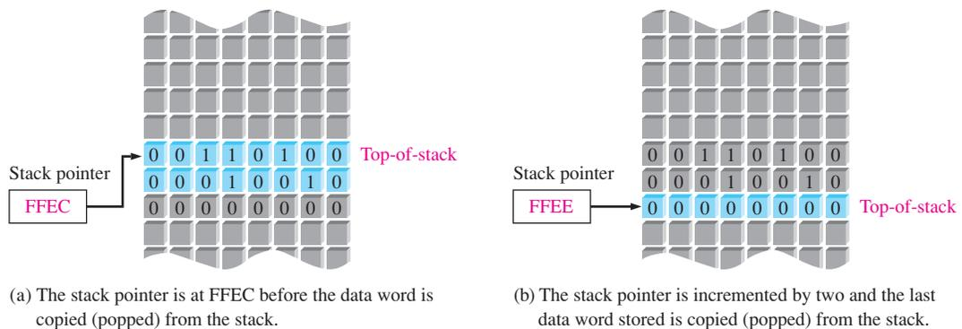
**FIGURE 11–57** Illustration of the POP operation for the RAM stack.
