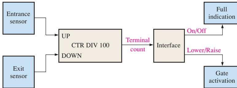
**FIGURE 9–51** Functional block diagram for parking garage control.
