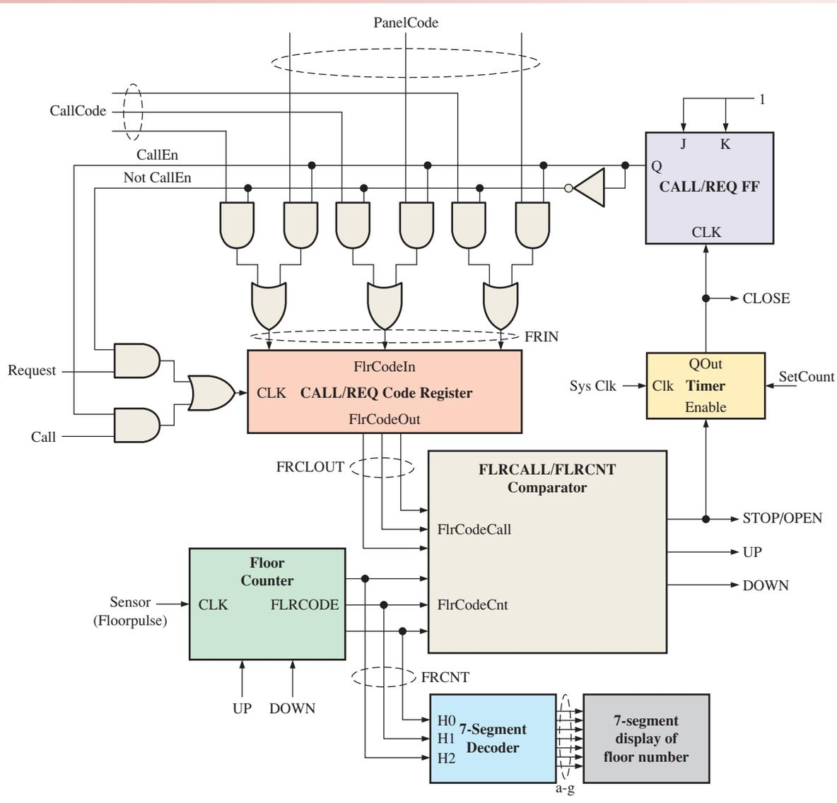
**FIGURE 10–62** Programming model of the elevator controller.
