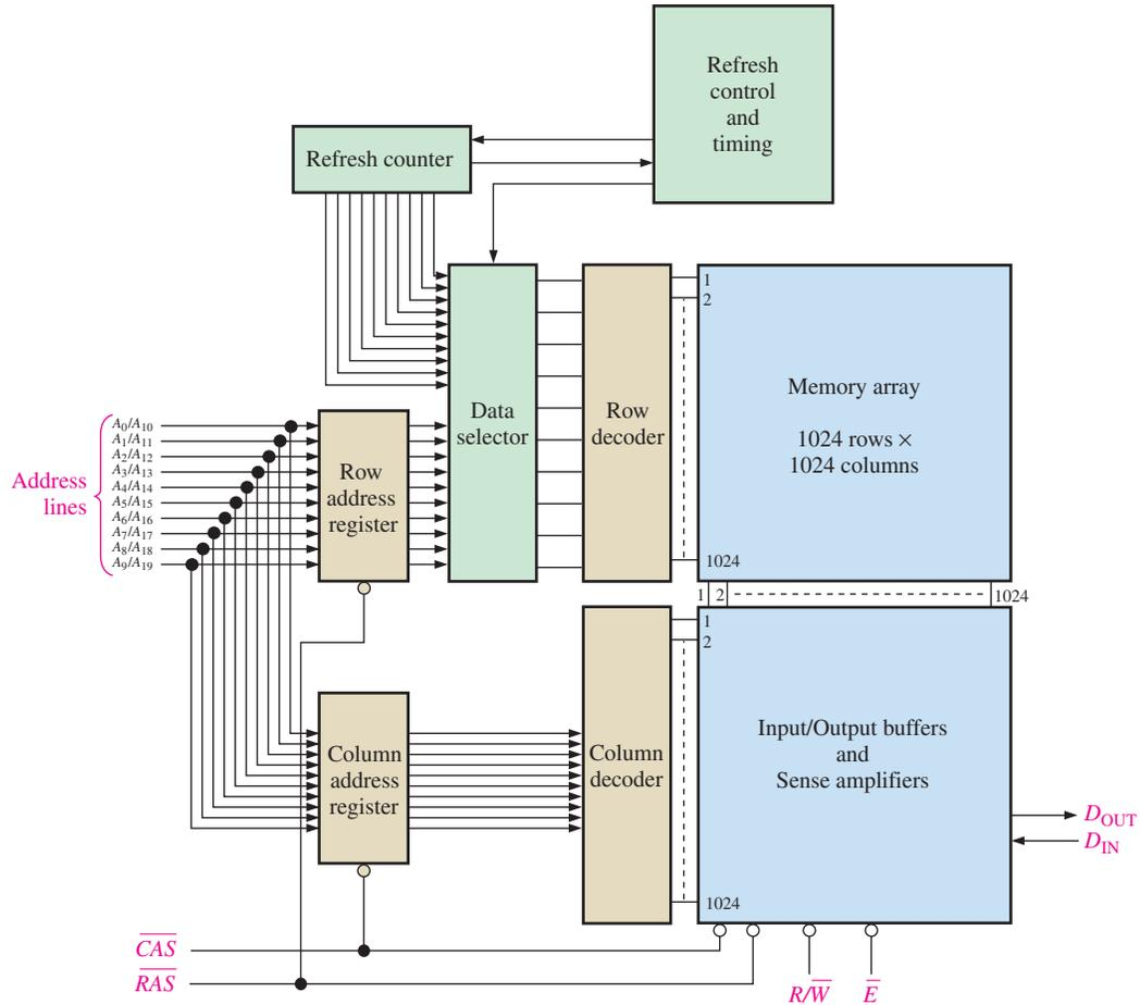
**FIGURE 11-19** Simplified block diagram of a 1M × 1 DRAM.
