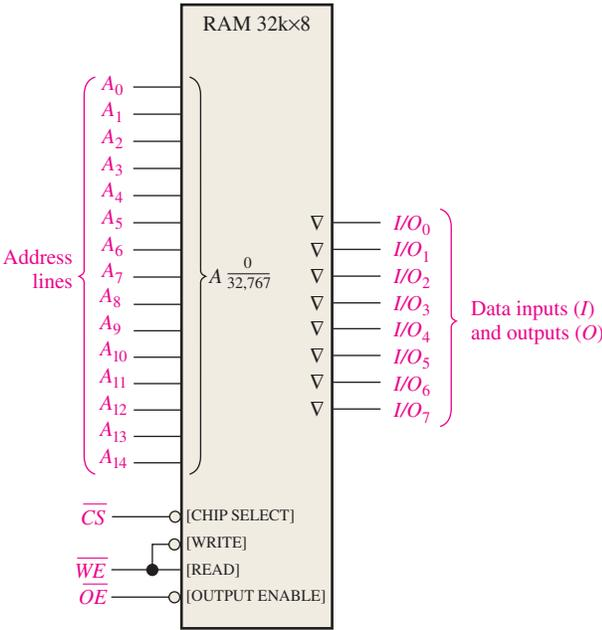
FIGURE 11-11 Logic diagram for an asynchronous 32k × 8 SRAM.
