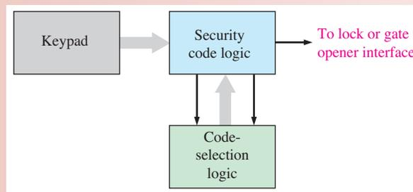
**FIGURE 8-42** Block diagram of the security system.
