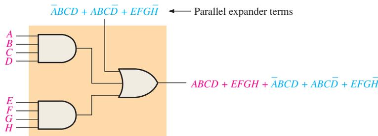
**FIGURE 10–13** Basic concept of the parallel expander.
