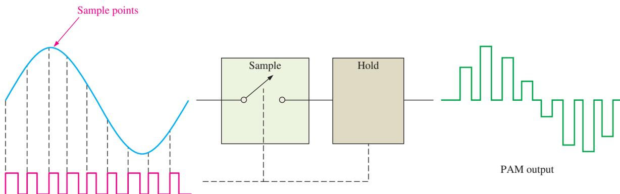
**FIGURE 13-28** Basic method of pulse amplitude modulation.
