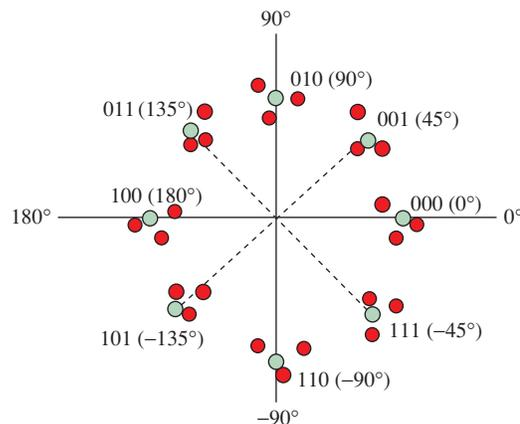
**FIGURE 13-25** Constellation map for a 3-bit PSK transmission. The phases are  $0^\circ$ ,  $45^\circ$ ,  $90^\circ$ ,  $135^\circ$ ,  $180^\circ$ ,  $-45^\circ$ ,  $-90^\circ$ , and  $-135^\circ$ , as indicated.
