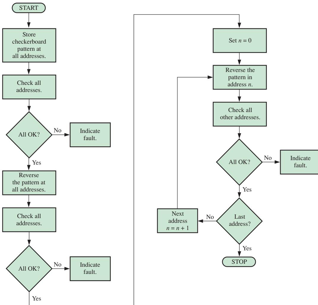
**FIGURE 11-77** Flowchart for basic RAM checkerboard test.
