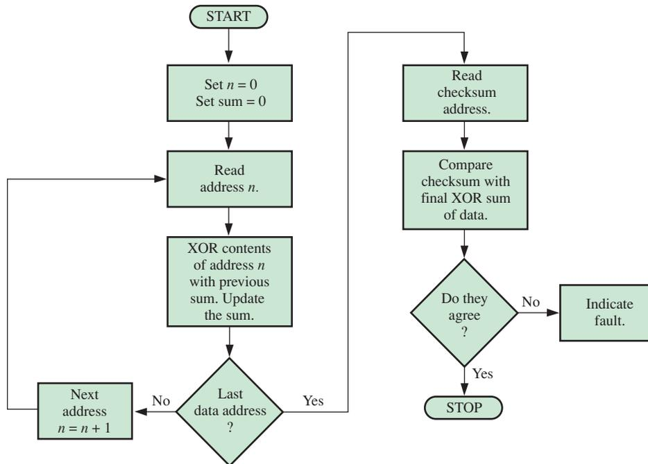
**FIGURE 11-75** Flowchart for a basic checksum test.
