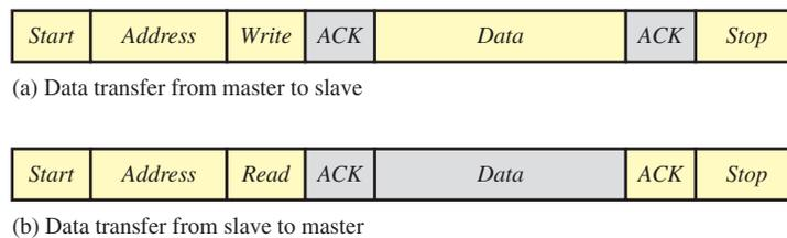
**FIGURE 13-70** I<sup>2</sup>C data transfers. Yellow is from master. Gray is from slave.
