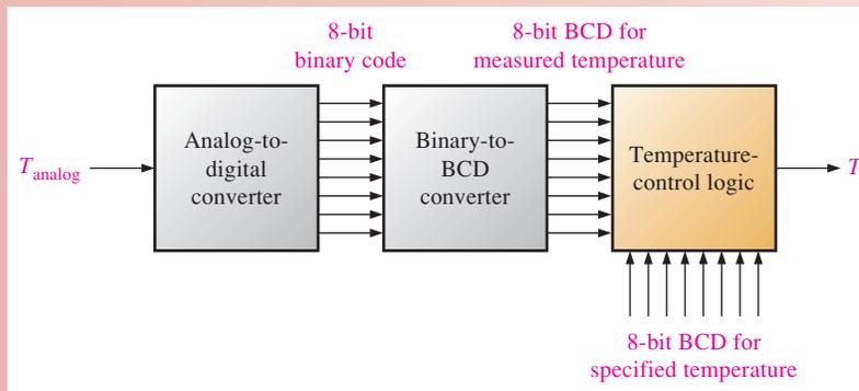
**FIGURE 5–51** Block diagram for temperature control circuit.
