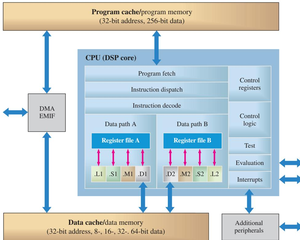
**FIGURE 12-40** General block diagram of the TMS320C6000 series DSP.
