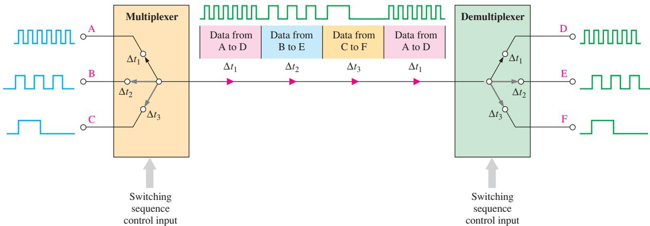
**FIGURE 1-24** Illustration of a basic multiplexing/demultiplexing application.
