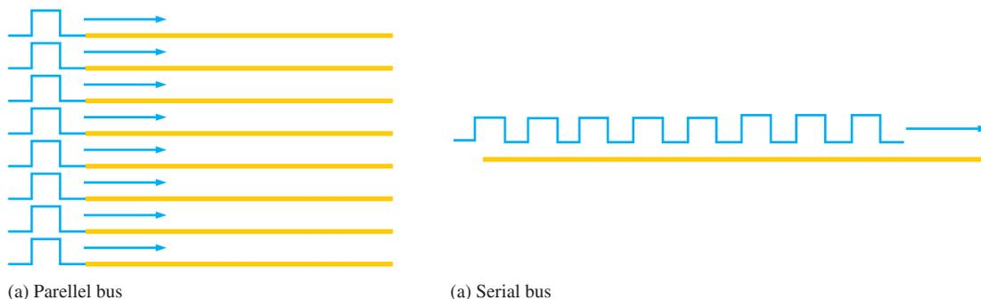
**FIGURE 13–51** Comparison of parallel and serial buses.
