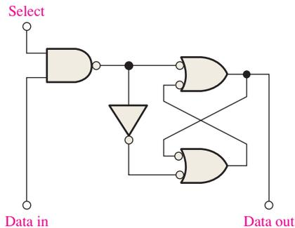
**FIGURE 11-9** A typical SRAM latch memory cell.
