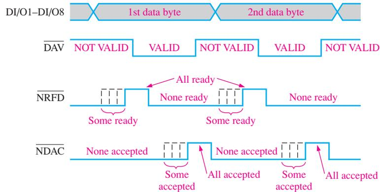
**FIGURE 13-59** Timing diagram for the GPIB handshaking sequence.
