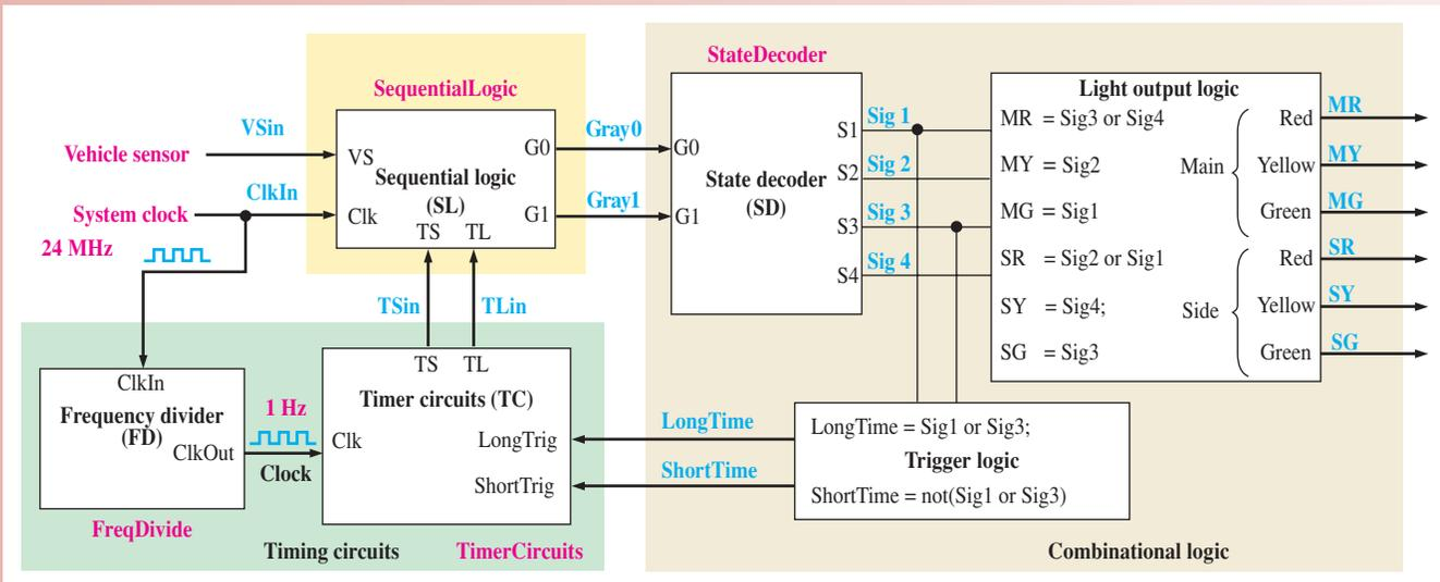
**FIGURE 7-66** Programming model for the traffic signal controller.
