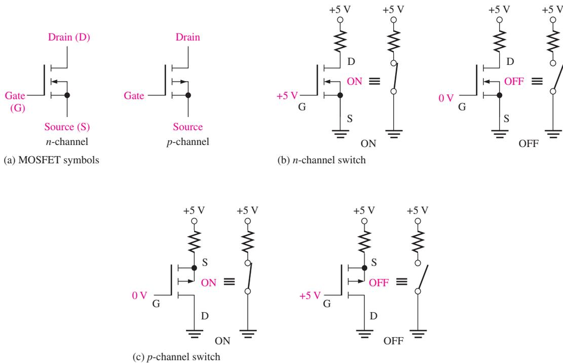
**FIGURE 15–15** Basic symbols and switching action of MOSFETs.
