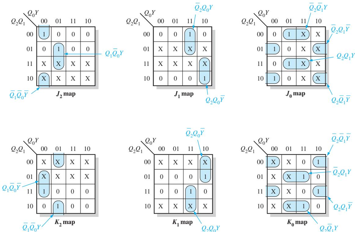
**FIGURE 9-34**  $J$  and  $K$  maps for Table 9–12. The UP/DOWN control input,  $Y$ , is treated as a fourth variable.
