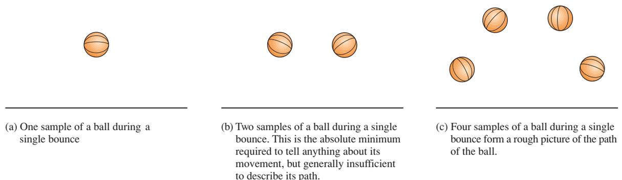
**FIGURE 12–2** Bouncing ball analogy of sampling theory.
