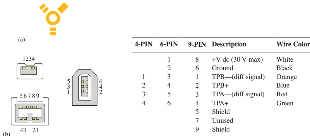
**FIGURE 13-73** Firewire symbol with cable and connector wires and pins.
