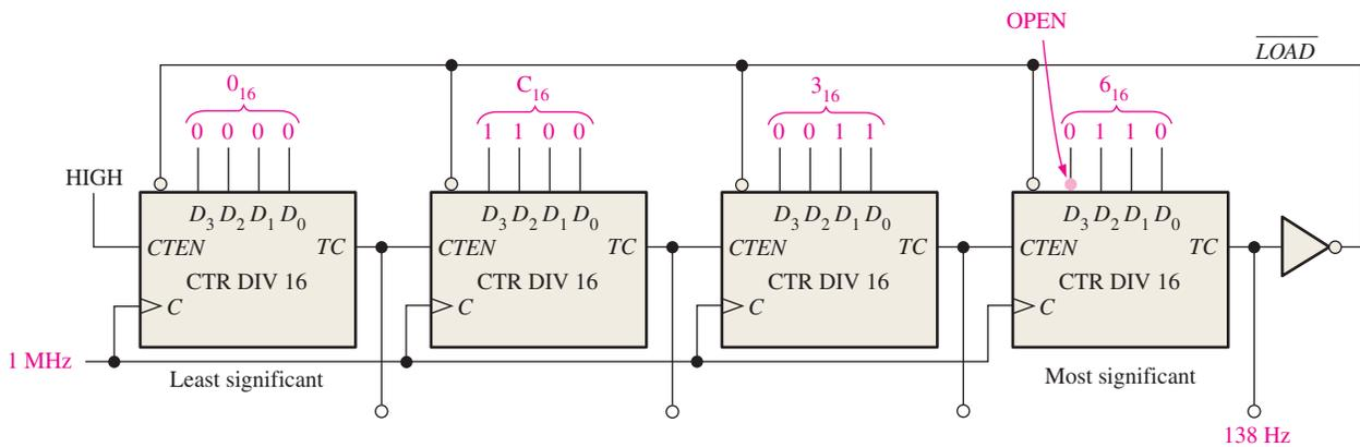
For example, suppose the  $D_3$  input of the most significant counter in Figure 9-57 is open and acts as a HIGH. Instead of  $6_{16}$  (0110) being preset into the counter,  $E_{16}$  (1110) is preset in. So, instead of beginning with  $63C0_{16}$  ( $25,536_{10}$ ) each time the counter recycles, the sequence will begin with  $E3C0_{16}$  ( $58,304_{10}$ ). This changes the modulus of the counter from 40,000 to  $65,536 - 58,304 = 7232$ .
