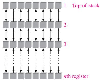
**FIGURE 11-52** Register stack.
