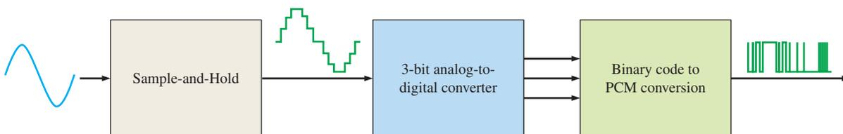
**FIGURE 13-38** Block diagram of a PCM system.
