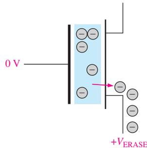
To erase a cell, a sufficient positive voltage is applied to the source with respect to the control gate to remove charge from the floating gate during the erase operation.
