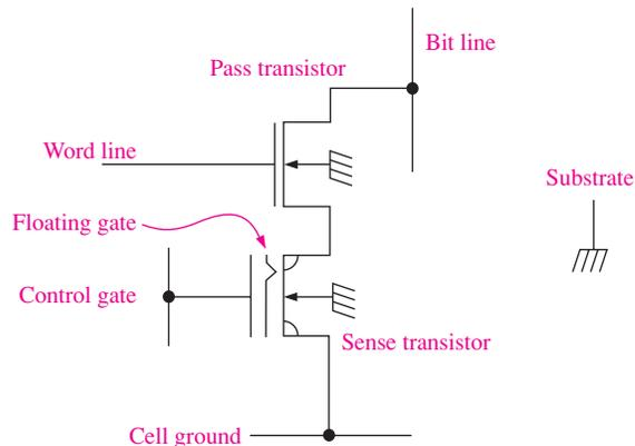
**FIGURE 15-49** An E<sup>2</sup>CMOS cell.
