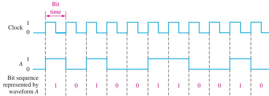
**FIGURE 1-11** Example of a clock waveform synchronized with a waveform representation of a sequence of bits.
