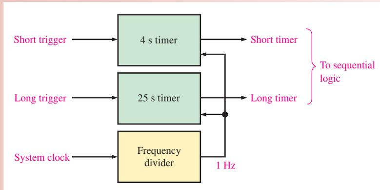
**FIGURE 7-65** Block diagram of the timing circuits unit.
