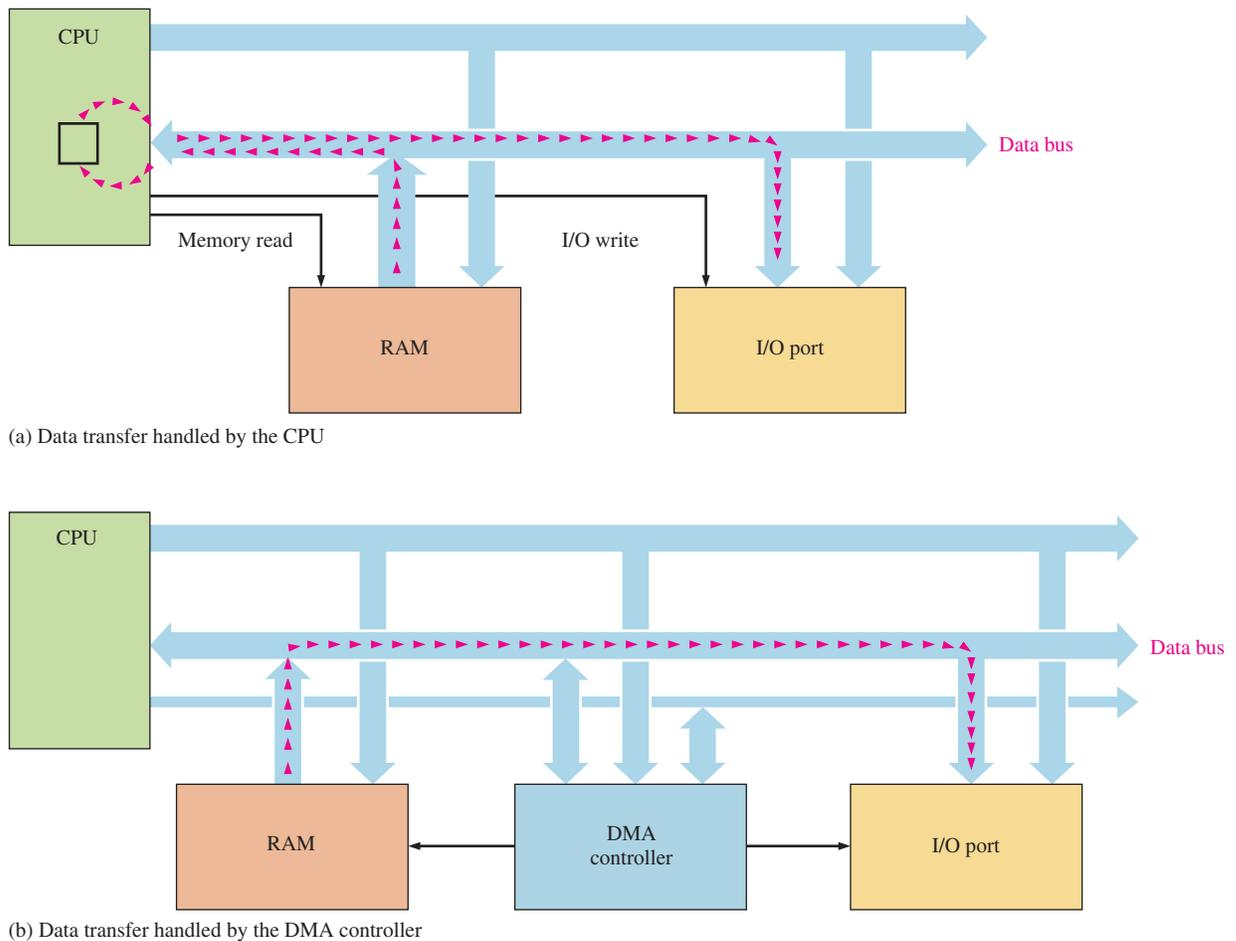
**FIGURE 14–24** Illustration of DMA vs CPU data transfer.
