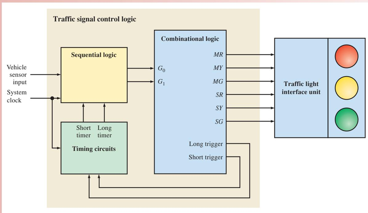
**FIGURE 7-64** Block diagram of the traffic signal controller.
