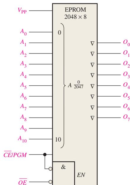
**FIGURE 11-31** The logic symbol for a  $2048 \times 8$  EPROM.
