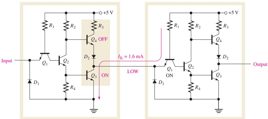
(b) Current sinking ( $I_{IL}$  value is maximum)
