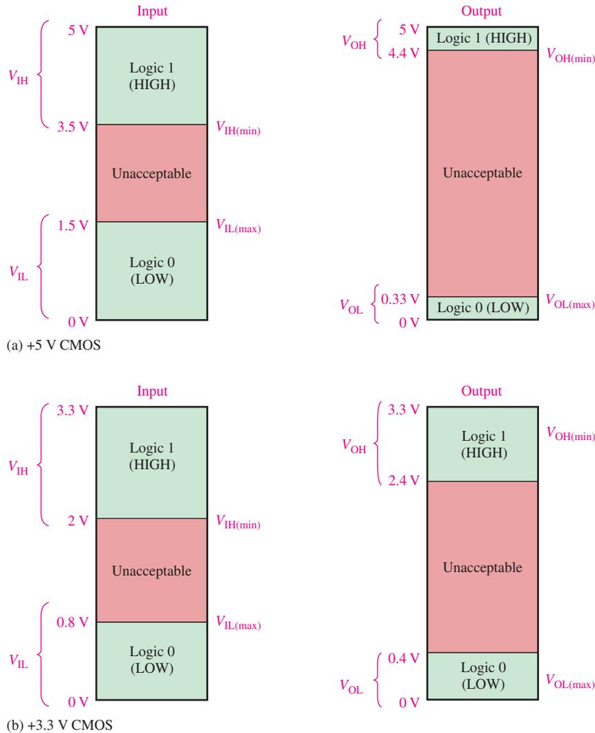
**FIGURE 15–2** Input and output logic levels for CMOS.
