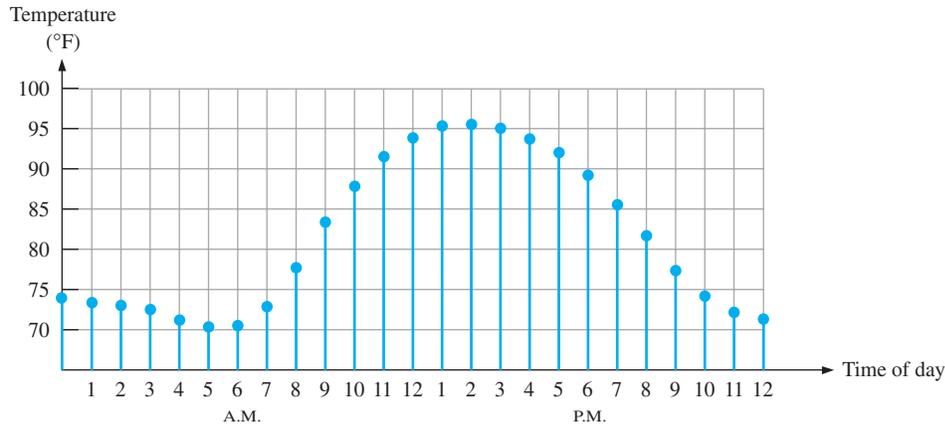
**FIGURE 1-2** Sampled-value representation (quantization) of the analog quantity in Figure 1-1. Each value represented by a dot can be digitized by representing it as a digital code that consists of a series of 1s and 0s.
