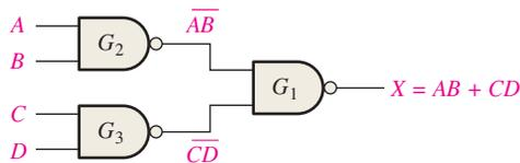
**FIGURE 5-20** NAND logic for  $X = AB + CD$ .
