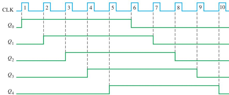
**FIGURE 8-23** Timing sequence for a 5-bit Johnson counter.
