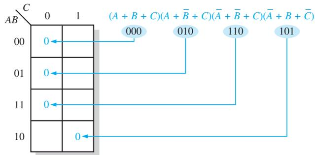
**FIGURE 4-43** Example of mapping a standard POS expression.
