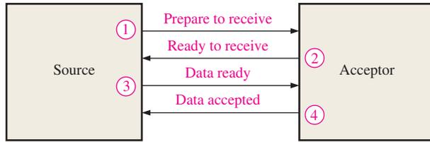
**FIGURE 13-75** An example of a handshaking sequence.
