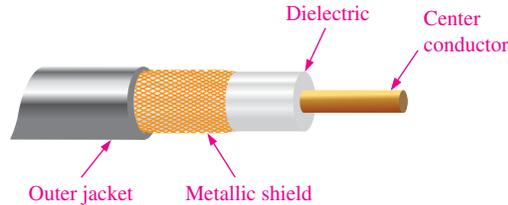
**FIGURE 13-3** Construction view of a coaxial cable.
