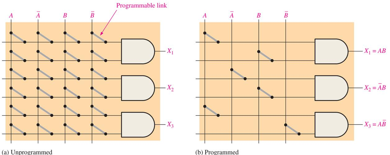
**FIGURE 3-49** Concept of a programmable AND array.
