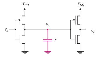
(b) The capacitive load at node A
