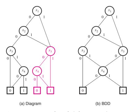
**Figure 8.24** Derivation of a BDD for the function in Example 8.11.
