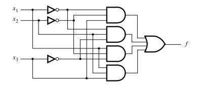
Figure PB.1 A sum-of-products CMOS circuit.
