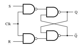
Figure 5.6 Gated SR latch with NAND gates.
