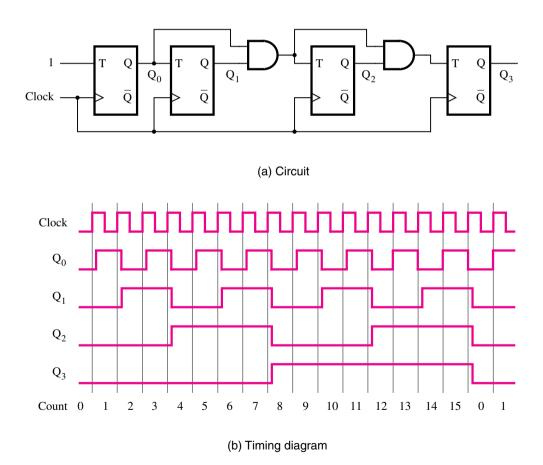
Figure 5.21 A four-bit synchronous up-counter.
