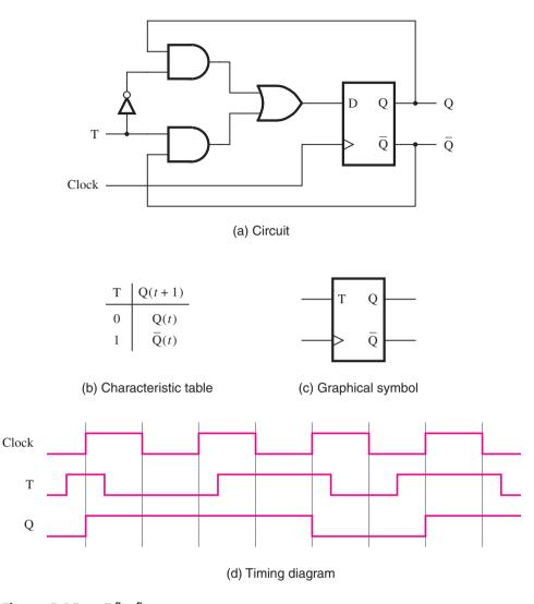
Figure 5.15 T flip-flop.
