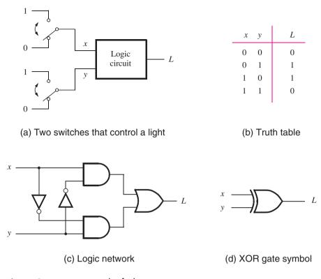
Figure 2.11 An example of a logic circuit.
