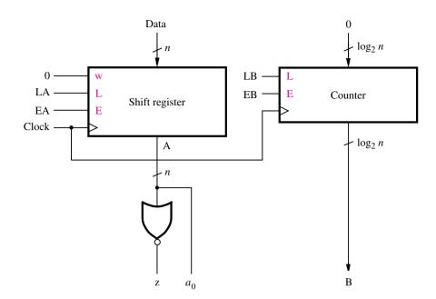
Figure 7.18 Datapath for the ASM chart in Figure 7.17.
