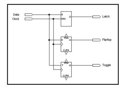
Figure 5.30 Three types of storage elements in a schematic.
