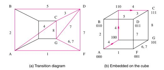
Figure 9.73 Determination of the state assignment.
