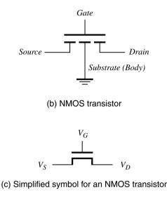
Figure B.2 NMOS transistor as a switch.
