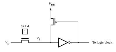
**Figure B.74** Restoring a high voltage level.
