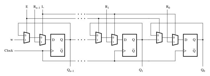
Figure 5.59 A shift register with parallel-load and enable control inputs.
