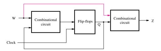
Figure 6.1 The general form of a sequential circuit.
