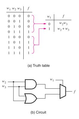
Figure 4.10 The three-input majority function implemented using a 2-to-1 multiplexer.
