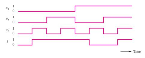
Figure P2.4 A timing diagram representing a logic function.
