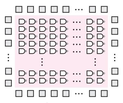
Figure B.41 A sea-of-gates gate array.
