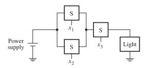
Figure 2.4 A series-parallel connection.
