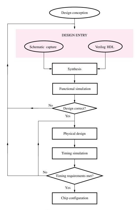
Figure 10.1 A typical CAD system.
