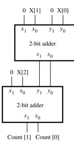
Figure A.15 A circuit that implements the code in Figure A.14.
