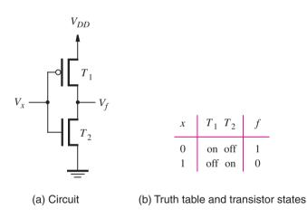
Figure B.12 CMOS realization of a NOT gate.
