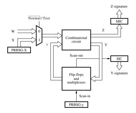
Figure 11.17 BIST in a sequential circuit.
