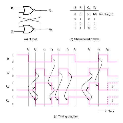
Figure 5.4 A basic latch built with NOR gates.
