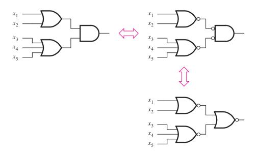
Figure 2.28 Using NOR gates to implement a product-of-sums.
