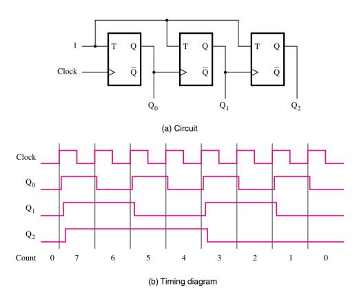
Figure 5.20 A three-bit down-counter.
