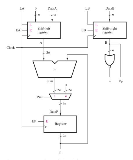
Figure 7.24 Datapath circuit for the multiplier.
