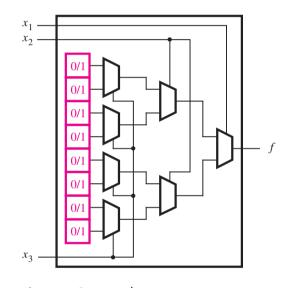
Figure B.37 A three-input LUT.
