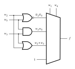
Figure 4.46 Circuit for Example 4.26.
