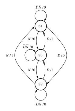
Figure 6.58 Mealy-type FSM for Example 6.7.
