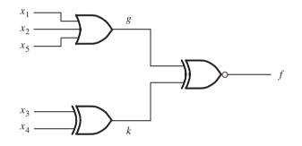
(b) Circuit obtained using decomposition
