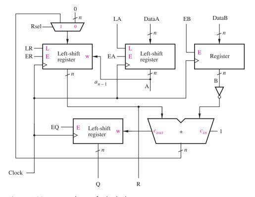
Figure 7.30 Datapath circuit for the divider.
