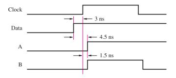
**Figure 7.49** Flip-flop timing in a chip.
