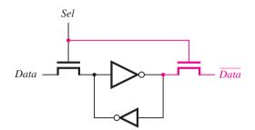
Figure B.64 An SRAM cell.
