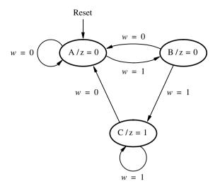
Figure A.37 State diagram of a simple Moore-type FSM.
