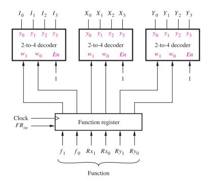
Figure 7.11 The function register and decoders.
