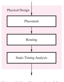
**Figure 10.7** Phases in physical design.
