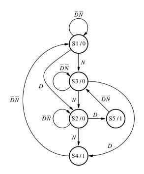
Figure 6.57 Minimized state diagram for Example 6.7.
