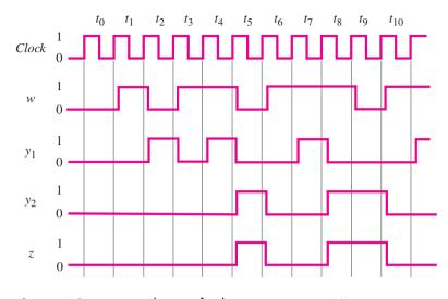
**Figure 6.9** Timing diagram for the circuit in Figure 6.8.
