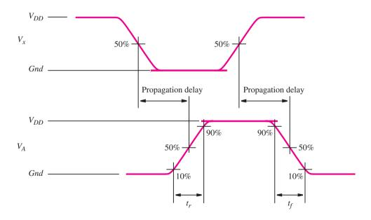
Figure B.48 Voltage waveforms for logic gates.
