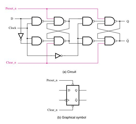
Figure 5.12 Master-slave D flip-flop with Clear and Preset.
