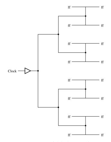
Figure 7.47 An H tree clock distribution network.
