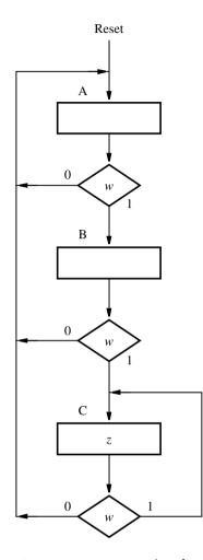
Figure 6.82 ASM chart for the FSM in Figure 6.3.
