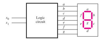
(a) Logic circuit and 7-segment display
