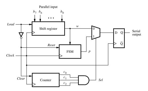
Figure 6.97 Parallel-to-serial converter.
