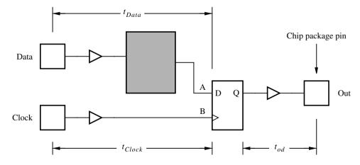
**Figure 7.48** A flip-flop in an integrated circuit chip.
