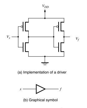
Figure B.60 A noninverting driver.
