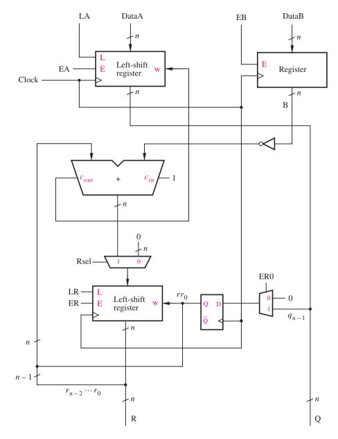
Figure 7.34 Datapath circuit for the enhanced divider.
