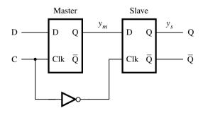
**Figure 9.5** Circuit for the master-slave D flip-flop.
