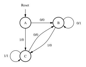
Figure 6.91 State diagram for Example 6.14.
