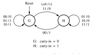
Figure 6.40 State diagram for the serial adder FSM.
