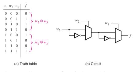
Figure 4.8 Three-input XOR implemented with 2-to-1 multiplexers.
