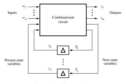
Figure 6.85 The general model for a sequential circuit.
