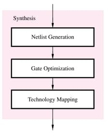
Figure 10.2 The stages included in a synthesis tool.
