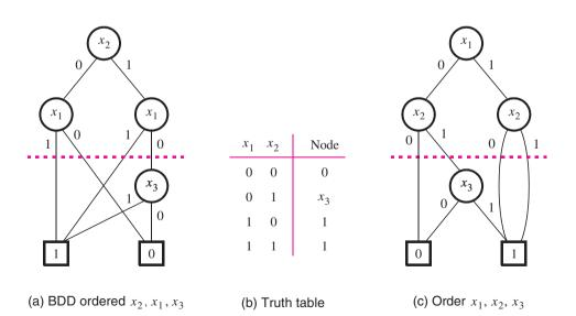
Figure 8.23 Reordering the nodes in a BDD.
