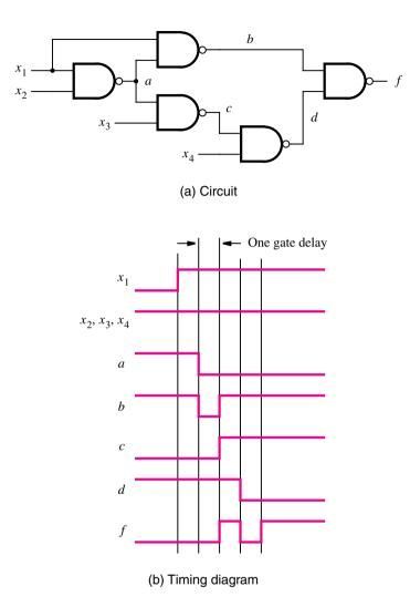
Figure 9.66 Circuit with a dynamic hazard.
