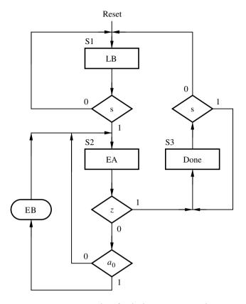
Figure 7.19 ASM chart for the bit counter control circuit.
