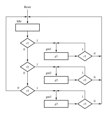
Figure 6.84 ASM chart for the arbiter FSM in Figure 6.73.
