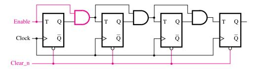
Figure 5.22 Inclusion of Enable and Clear capability.
