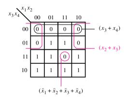
**Figure 2.61** POS minimization of  $f(x_1, ..., x_4) = \Pi M(0, 1, 4, 8, 9, 12, 15).$
