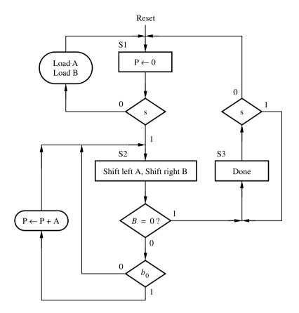
Figure 7.23 ASM chart for the multiplier.
