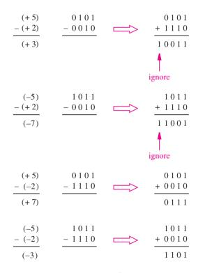
Figure 3.10 Examples of 2's complement subtraction.
