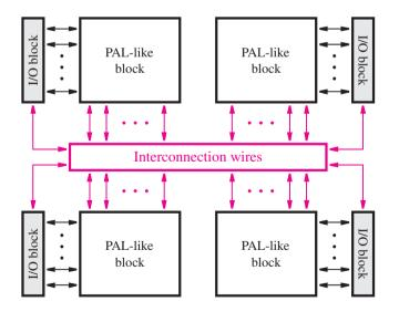
Figure B.32 Structure of a complex programmable logic device (CPLD).
