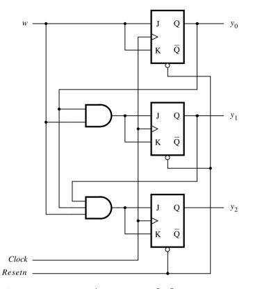
Figure 6.67 Circuit diagram using JK flip-flops.
