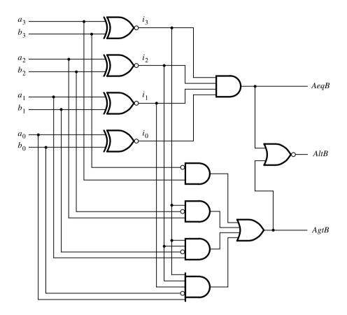
Figure 4.22 A four-bit comparator circuit.
