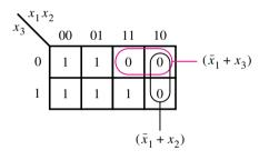
**Figure 2.60** POS minimization of  $f(x_1, x_2, x_3) = \Pi M(4, 5, 6)$ .
