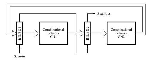
Figure 11.19 Using BILBO circuits for testing.
