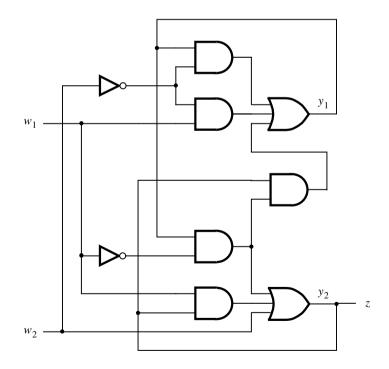
Figure 9.76 Circuit for Example 9.19.
