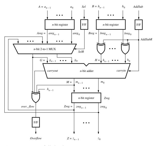
Figure 10.4 Circuit specified by the code in Figure 10.3.
