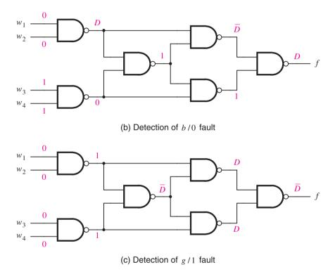
Figure 11.4 Detection of faults.
