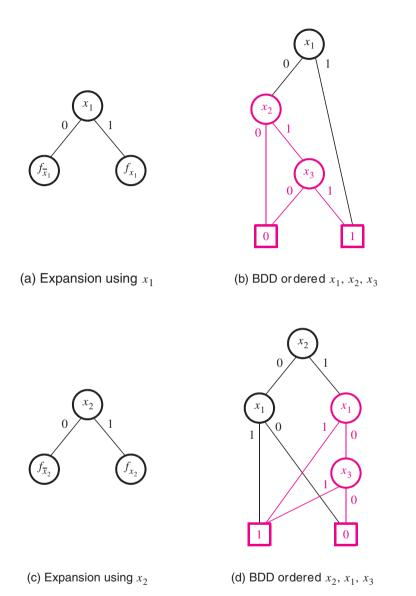
**Figure 8.22** Derivation of BDDs for  $f = x_1 + x_2 x_3$ .
