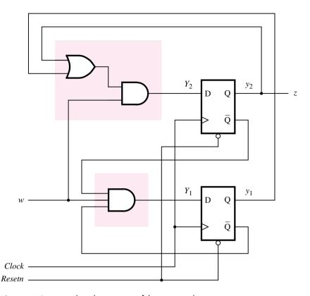
**Figure 6.8** Final implementation of the sequential circuit.
