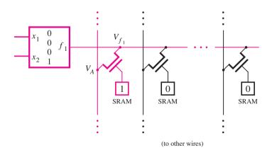
Figure B.73 Pass-transistor switches in FPGAs.
