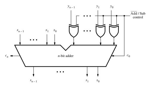
Figure 3.12 Adder/subtractor unit.
