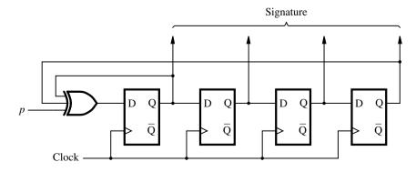
Figure 11.15 Single-input compressor circuit (SIC).
