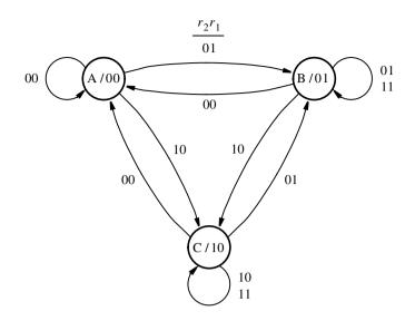
Figure 9.20 State diagram for the arbiter.
