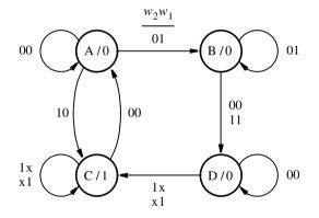
**Figure 9.11** State diagram for Example 9.3.
