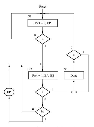
Figure 7.25 ASM chart for the multiplier control circuit.
