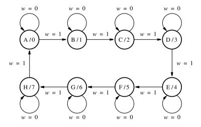
Figure 6.60 State diagram for the counter.
