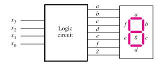
(a) Logic circuit and 7-segment display
