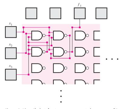
**Figure B.42** The logic function  $f_1 = x_2 \overline{x}_3 + x_1 x_3$  in the gate array of Figure B.41.
