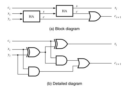
Figure 3.4 A decomposed implementation of the full-adder circuit.
