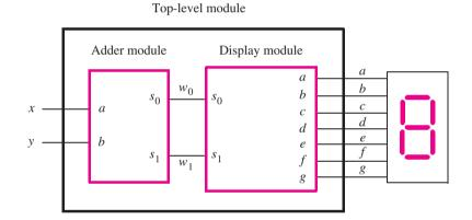
Figure 2.44 A logic circuit with two modules.
