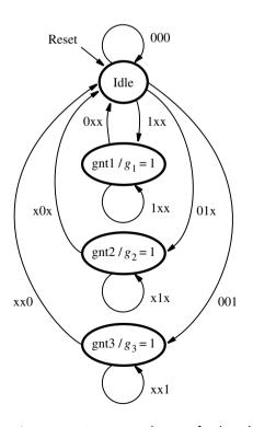
Figure 6.72 State diagram for the arbiter.
