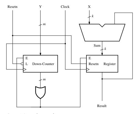
**Figure A.35** The accumulator circuit.
