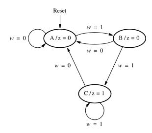
**Figure 6.3** State diagram of a simple sequential circuit.
