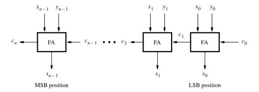
**Figure 3.5** An *n*-bit ripple-carry adder.
