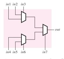
Figure PB.9 A gate-array logic cell.
