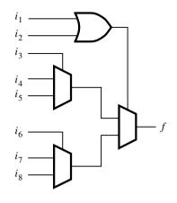
Figure P4.1 A multiplexer-based circuit.
