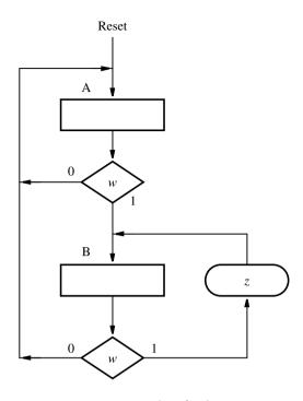
Figure 6.83 ASM chart for the FSM in Figure 6.23.
