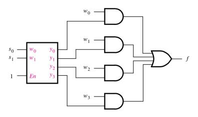
Figure 4.17 A 4-to-1 multiplexer built using a decoder.
