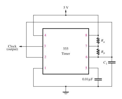
Figure P7.2 The 555 programmable timer chip.
