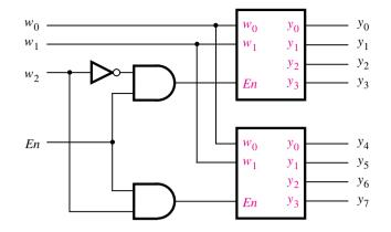
Figure 4.15 A 3-to-8 decoder using two 2-to-4 decoders.
