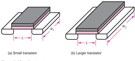
Figure B.49 Transistor sizes.
