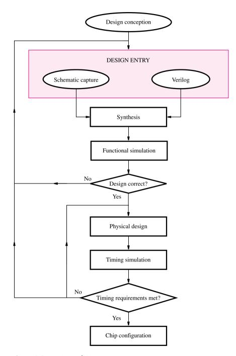
Figure 2.35 A typical CAD system.
