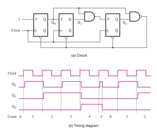
Figure 5.26 A modulo-6 counter with asynchronous reset.
