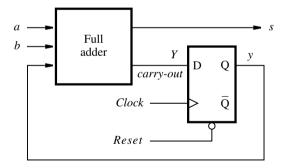
Figure 6.43 Circuit for the adder FSM in Figure 6.39.
