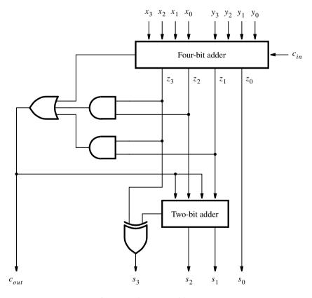
**Figure 3.41** Circuit for a one-digit BCD adder.
