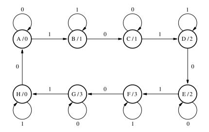
Figure 9.17 State diagram for a modulo-4 counter.
