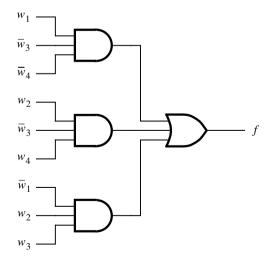
Figure 11.5 Circuit with a tree structure.
