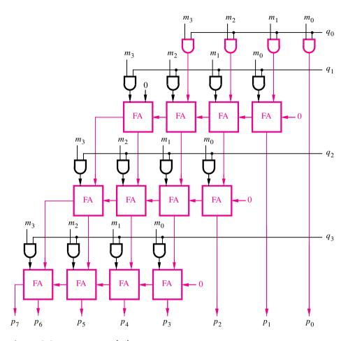
**Figure 3.35** A 4 × 4 multiplier circuit.
