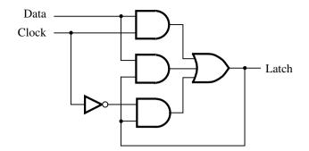
Figure 5.31 Gated D latch generated by CAD tools.
