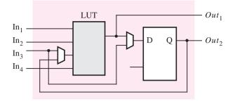
(a) An FPGA logic element.
