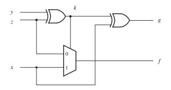
Figure 2.70 The logic circuit for Example 2.29.
