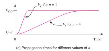
**Figure B.59** The effect of fan-out on propagation delay.
