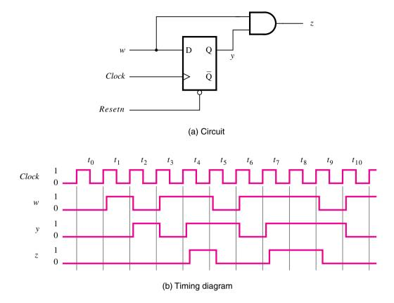
Figure 6.26 Implementation of the FSM in Figure 6.25.
