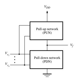
Figure B.11 Structure of a CMOS circuit.
