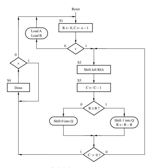
Figure 7.29 ASM chart for the divider.
