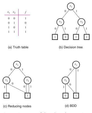
Figure 8.19 Derivation of a binary decision diagram (BDD).
