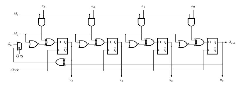
Figure 11.18 A four-bit built-in logic block observer (BILBO).
