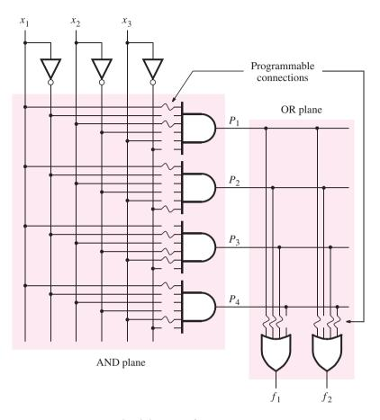
Figure B.26 Gate-level diagram of a PLA.
