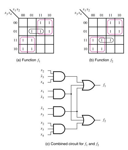
Figure 2.64 An example of multiple-output synthesis.
