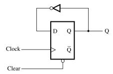
**Figure 5.66** A simple flip-flop circuit.
