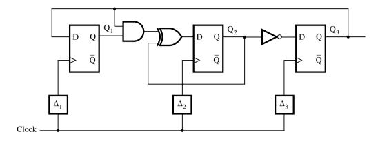
Figure 5.76 A circuit with clock skews.
