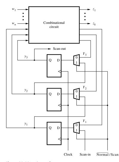
Figure 11.11 Scan-path arrangement.
