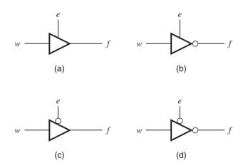
Figure B.62 Four types of tri-state drivers.
