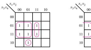
(c) Optimal realization of  $f_{\rm 3}$  and  $f_{\rm 4}$  together
