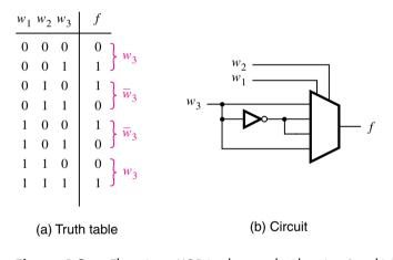
Figure 4.9 Three-input XOR implemented with a 4-to-1 multiplexer.
