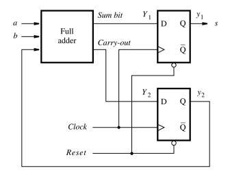
Figure 6.47 Circuit for the Moore-type serial adder FSM.
