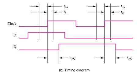
Figure 5.14 Flip-flop timing parameters.
