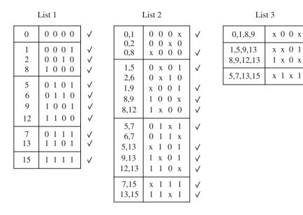
**Figure 8.27** Generation of prime implicants for the function in Example 8.12.
