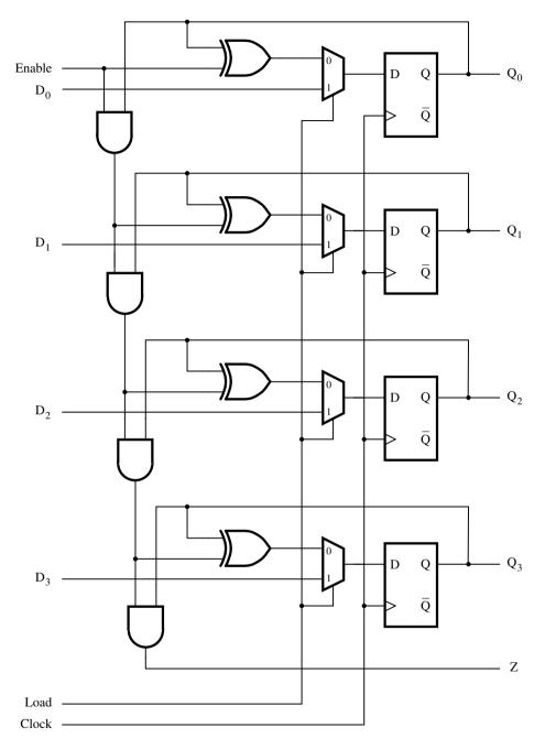
Figure 5.24 A counter with parallel-load capability.
