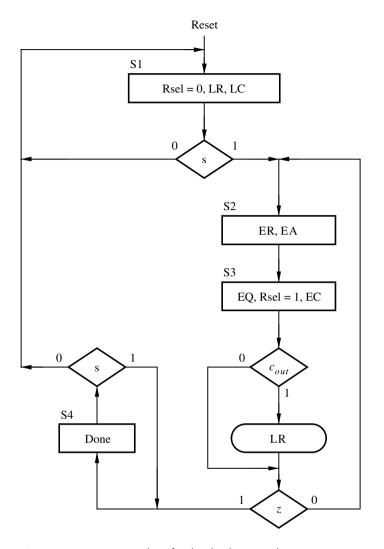
Figure 7.31 ASM chart for the divider control circuit.
