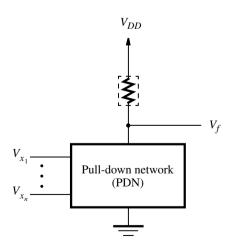
Figure B.10 Structure of an NMOS circuit.
