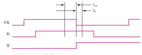
**Figure 5.8** Setup and hold times.
