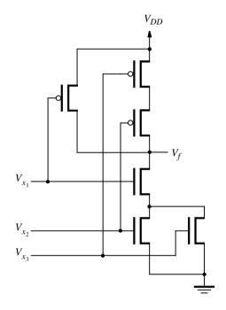
Figure PB.4 A three-input CMOS circuit.
