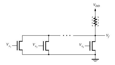
Figure B.58 High fan-in NMOS NOR gate.
