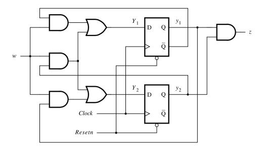
Figure 6.75 Circuit for Example 6.9.
