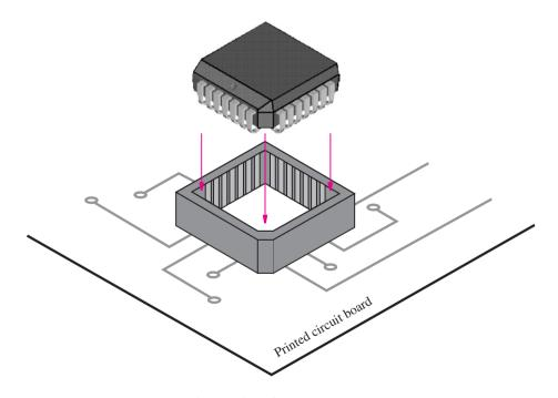
Figure B.31 A PLCC package with socket.
