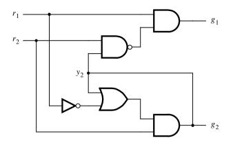
Figure 9.22 The arbiter circuit.
