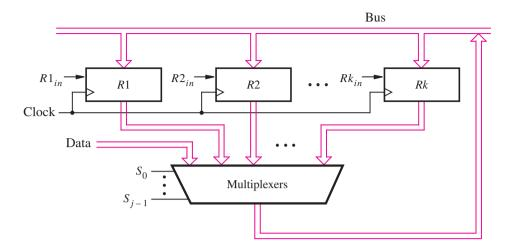
Figure 7.4 Using multiplexers to implement a bus.
