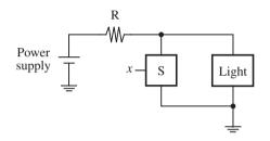
Figure 2.5 An inverting circuit.
