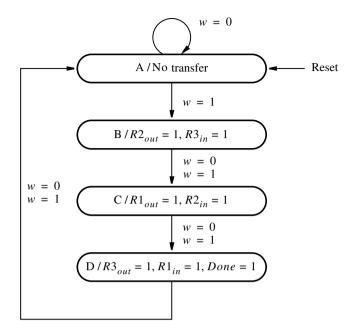
Figure 6.11 State diagram for Example 6.1.
