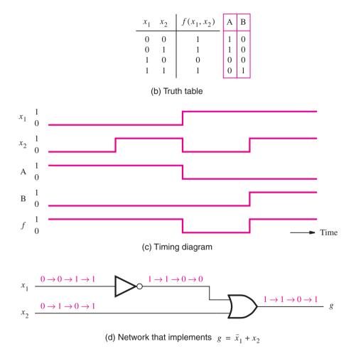
Figure 2.10 An example of logic networks.
