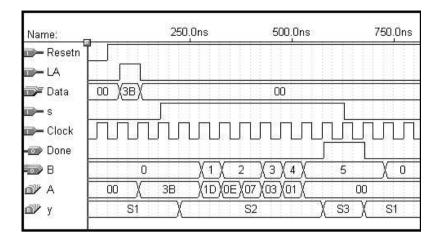
Figure 7.21 Simulation results for the bit-counting circuit.
