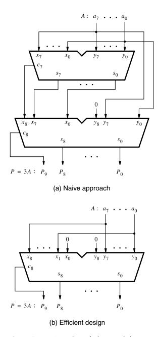
Figure 3.6 Circuit that multiplies an eight-bit unsigned number by 3.
