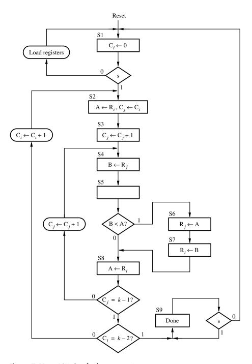
Figure 7.41 ASM chart for the sort operation.
