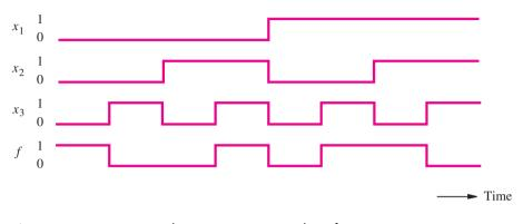
Figure P2.3 A timing diagram representing a logic function.
