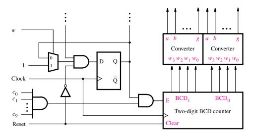
Figure 5.69 A modified version of the reaction-timer circuit.
