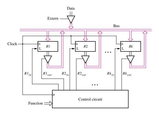
**Figure 7.2** A digital system with k registers.
