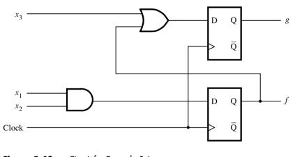
Figure 5.43 Circuit for Example 5.6.
