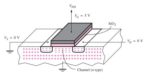
(b) When  $V_{GS}$  = 5 V, the transistor is on
