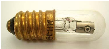
Figure 9. A gas discharge tube with a radioactive ioniser to aid starting.
