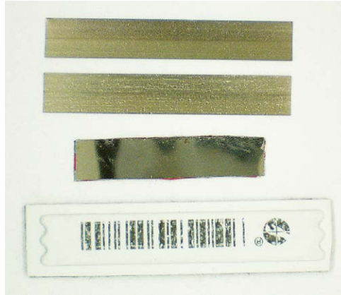
Figure 1. The AM label components, shown here are two resonators and a (shorter) magnetic strip.
