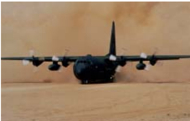
Fig. 27-8. A C-130 Hercules taking off somewhere in the Kuwaiti Theater of Operations during the Persian Gulf War. The original design of the C-130 dates from 1951. The rugged construction of these aircraft allows them to use unprepared runways, as are found forward on the battlefield. Photograph: Defense Audio-Visual Agency, Still Media Depository, Washington, DC.
