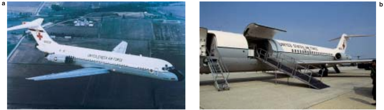
Fig. 27-12. The C-9 Nightingale (a), a modified version of the commercial DC-9 and the only US Air Force aircraft especially designed for aeromedical evacuation. (b) The loading ramp. Photographs: Courtesy of Lieutenant Colonel Charles Beading, MD, Medical Corps, US Air Force, Flight Surgeon, Uniformed Services University of the Health Sciences, Bethesda, Md.
