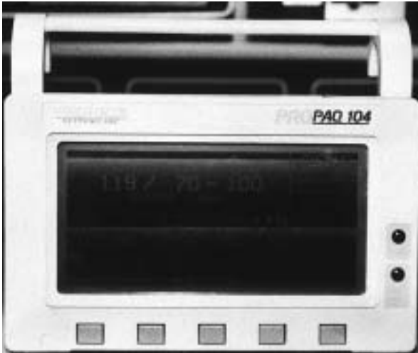
Fig. 5-1. This patient monitor, the PROPAC 104 (portable anesthesia circuit, manufactured by Protocol Systems, Inc., Beaverton, Ore.), has ports for noninvasive measurement of arterial blood pressure, electrical activity of the heart, and temperature, and has two additional pressure ports.
