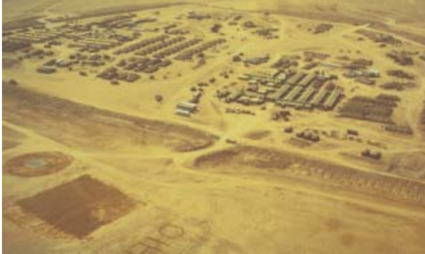
Fig. 6-11. Two evacuation hospitals, the 148th in the distance on the left and the 410th in the near right, deployed in the Kuwaiti Theater of Operations during the Persian Gulf War. TEMPER tents form much of the central portion of the 410th. ISO shelters can be identified by their lighter color. Hospital personnel are billeted in the complex of canvas tents that occupy the right side of the hospital. TEMPER: tents, extendable, modular, personnel; ISO: International Standards Organization. Photograph: Courtesy of Public Affairs, Office of The Surgeon General, US Army.
