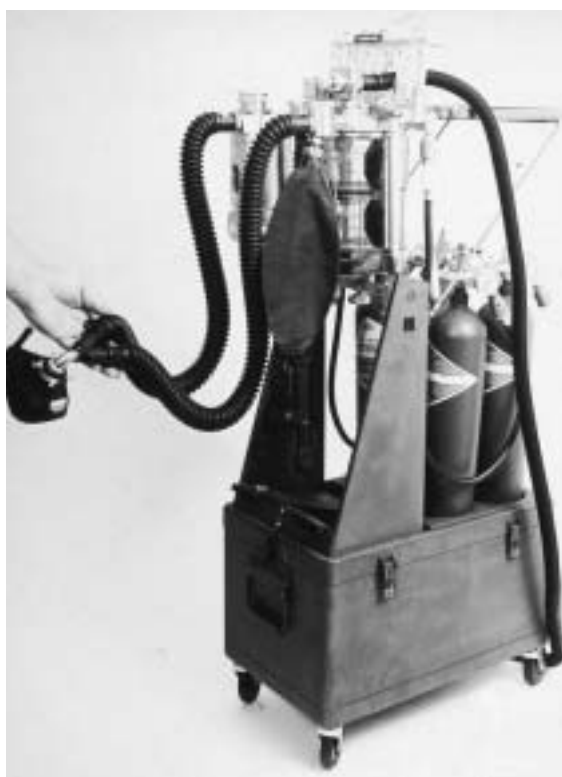
Fig. 7-36. The Field Anesthesia Machine (FAM) Model 885A is configured with an adult breathing circuit. A corrugated hose is attached to the scavenger port of the pop-off valve. The inspiratory limb of the breathing circuit is attached to the outlet port near the vaporizer, and the expiratory limb is attached to the inlet port near the exhalation valve. Photograph: Printed with permission from Ohmeda, Inc, Madison, Wis.
