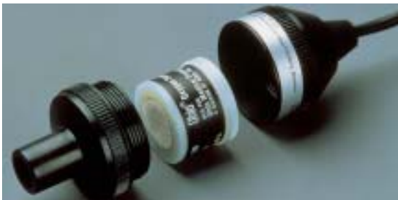
Fig. 7-47. An oxygen sensor housing showing the galvanic cell sensor cartridge. A cable from the housing connects the cartridge to the processor in the monitor, and the opposite end is placed in the tee of the inspiratory limb of the breathing circuit. Photograph: Printed with permission of Ohmeda, Inc, Madison, Wis.
