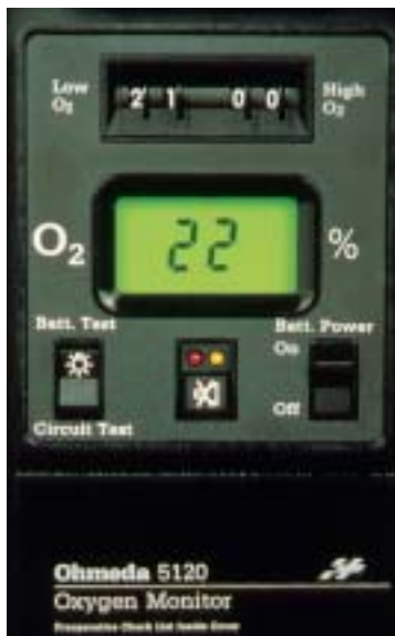
Fig. 7-49. An oxygen display of the percentage of oxygen in the gas mixture. Low-concentration and high-concentration alarms can be used by the anesthesia provider as conditions warrant. Photograph: Printed with permission of Ohmeda, Inc, Madison, Wis.
