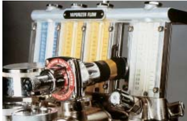
Fig. 7-30. The metabolic oxygen flowmeter control knob is fluted, labeled O 2 , painted white (international color assigned to oxygen), and is positioned on the far right. The flow-tube scale is labeled O 2 , ranges from 0.2 to 7 L/min, is also white, and is protected by a plastic shield. The adjustable pressure-limiting (pop-off) valve can be seen, with the proximal end of the scavenger hose attached.
