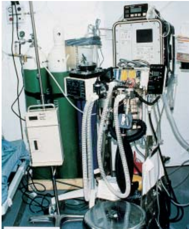
Fig. 7-25. Anesthesia equipment at the 12th Evacuation Hospital in Saudi Arabia during the Persian Gulf War. Patient monitors, a Field Anesthesia Machine (FAM) Model 885A with an oxygen monitor, a ventilator, and a blood warmer are shown. The rebreathing bag is attached to a switch-over valve that simplifies the adaptation of the ventilator to the breathing circuit. Against the wall (left) are two H-cylinders of compressed oxygen. These cylinders are painted two colors: green (US designation for oxygen) and white (international color assigned to oxygen), and are stamped OXYGEN in white letters on the green section of the cylinder. One oxygen H-cylinder is being used to power the ventilator, and the adapter and pin index safety system (PISS) regulator provided with the FAM are not being used. Nonstandard breathing tubes are connected to the FAM. Photograph: Courtesy of Captain DJ Rutkowski, CRNA, US Army Nurse Corps.
