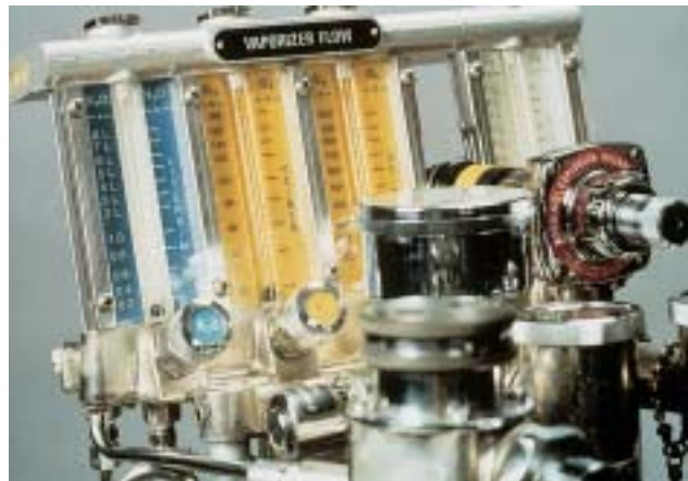
Fig. 7-31. Nitrous oxide and oxygen-for-vaporizer flowmeter control knobs and flow tubes. Nitrous oxide is labeled N 2 O and is painted blue (international and US color assigned to nitrous oxide). The nitrous oxide-flow-tube scale is labeled N 2 O, ranges from 0.2 to 8 L/min, is painted blue, and is protected by a plastic shield. The oxygen-for-vaporizer control knob is painted yellow (manufacturer's choice), and is labeled O 2 FOR VAPORIZER. The single oxygen-for-vaporizer flowmeter control knob meters both low- and high-flow oxygen. The flow-tube scales are labeled O 2 , painted yellow, and protected by a plastic shield; the low-flow tube ranges from 20 to 180 cc/min, and the high-flow tube ranges from 100 to 1,000 cc/min. The nitrous oxide pressure-sensor shutoff valve can be seen below the nitrous oxide flowmeter housing.
